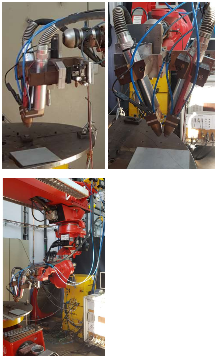
Figure 2. Tandem PTA with handling system (TU Chemnitz).
