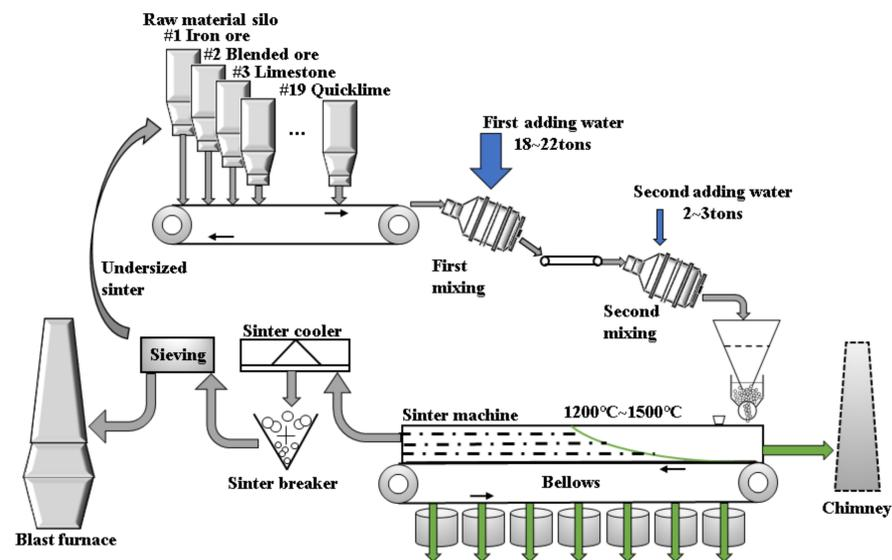
Figure 1. Sintering process layout diagram.
