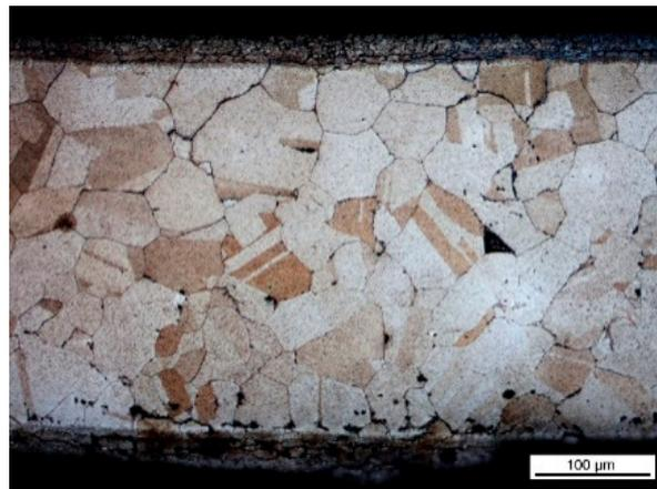
**Figure 5.** The ancient silver sample (of the silver bowl excavated in Yiwu City) was etched by diluted aqua regia (6 mL HCl + 2 mL  $\text{HNO}_3$  and diluted to 12 mL); etching duration: 15 s; impurity removal: 1 mol/L sodium thiosulfate solution for 60 s.
