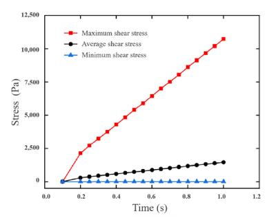
Figure 19. Variation of wall shear stress on the stent, with time, in a single cycle.
