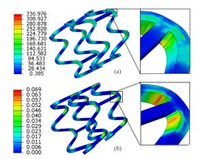
Figure 10. The equivalent stress (a) and equivalent strain (b) distribution of the stent after spring-back.
