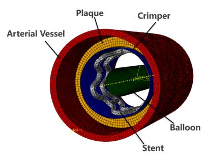
Figure 3. The mesh of L-type coronary artery stent coupling system.
