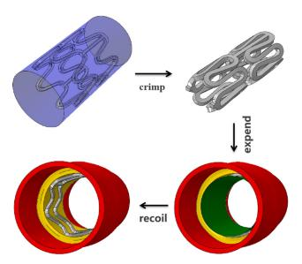
Figure 4. The displacement loading process of a coronary artery stent.
