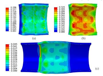
**Figure 13.** Distribution of equivalent stress (a), displacement (b), and equivalent stress (c) along the arterial wall after expansion of the stent.
