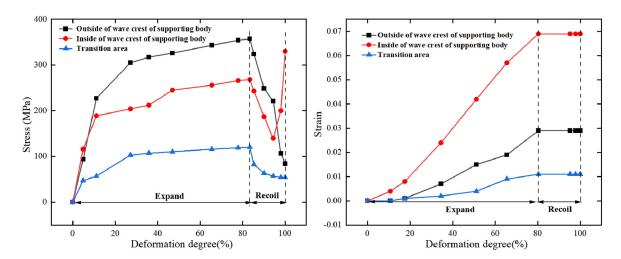
**Figure 11.** Variation of stress and strain at some points of L-type coronary stent during expansion stage.
