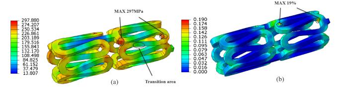
Figure 6. The equivalent stress (a) and equivalent strain (b) distribution clouds for the stent after crimping.
