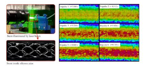
**Figure 16.** Blood velocity distribution in the vessel after coronary stent implantation Reproduced with permission from [37], Copyright 2020 Elsevier.
