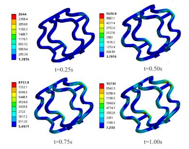
Figure 18. Distribution of wall shear stress (Pa) on the stent at different times.
