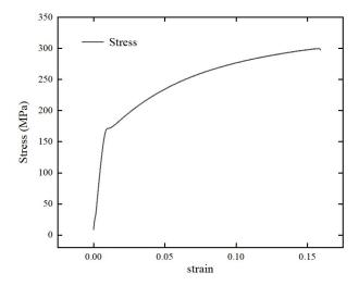
**Figure 1.** Tensile stress–strain curve for a Mg alloy (AZ31B).
