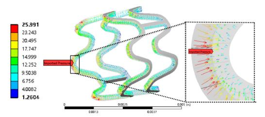
Figure 17. Pressure distribution of blood acting on the coronary artery stent at the maximum moment.
