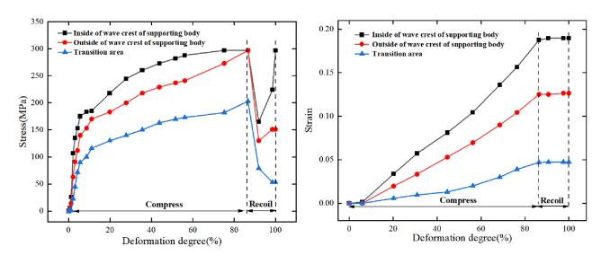
**Figure 8.** Variation of stress and strain at some points of L-type coronary stent during compression stage.
