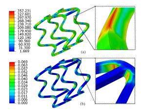
**Figure 9.** The equivalent stress (**a**) and equivalent strain (**b**) distribution of stent at the end of expansion.
