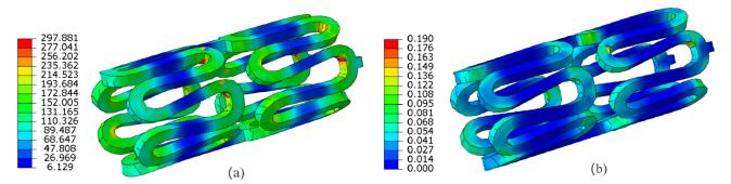
Figure 7. The equivalent stress (a) and equivalent strain (b) distribution contours for the stent after spring-back.
