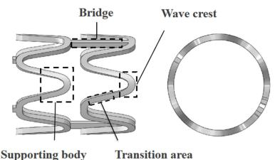
Figure 2. 3D model of Biotech's L-type coronary artery stent.
