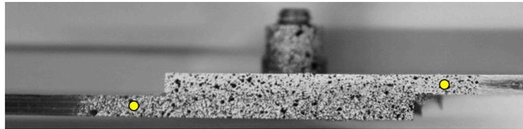
**Figure 6.** Example of a bonded/bolted specimen (overlap length: 26 mm and height: 4.55 mm) with a speckle pattern; the tracked points are shown in yellow and the displacement reported for each specimen was the magnitude of the vector between the points.
