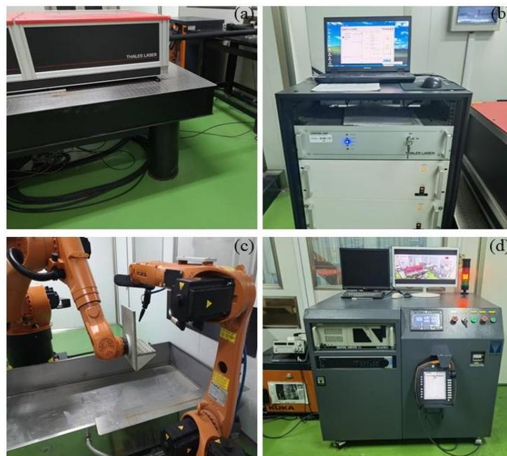
**Figure 3.** GAIA nanosecond pulse laser shock system: (a) laser system, (b) computer-integrated control system, (c) workbench and (d) path control system.
