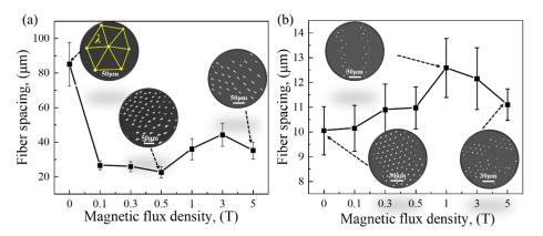
**Figure 3.** The fiber spacings ( $\lambda$ ) on the transverse sections of ingots directionally solidified under various MFDs at growth rates of 1  $\mu$ m/s ( $\bf a$ ) and 5  $\mu$ m/s ( $\bf b$ ), respectively.
