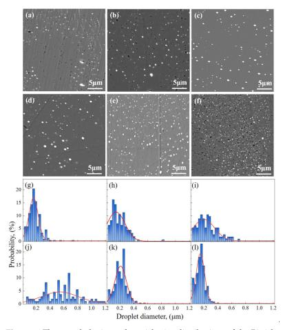
Figure 4. The morphologies and particle size distributions of the Bi-rich phases ahead of the S-L interface in the case of the growth rate of 5  $\mu$ m/s under various MFDs. (a,g) 0 T; (b,h) 0.1 T; (c,i) 0.5 T; (d,j) 1 T; (e,k) 3 T; (f,l) 5 T. (a–f) The morphologies of Bi-rich droplets ahead of the S-L interface under various MFDs. (g–l) The size distributions of Bi-rich droplets ahead of the S-L interface under various MFDs.
