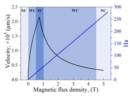
**Figure 6.** The curves of melt velocity caused by the TEMC and Ha numbers under various MFDs. NC, WC, and SC represent three different intensities of melt convection, respectively.
