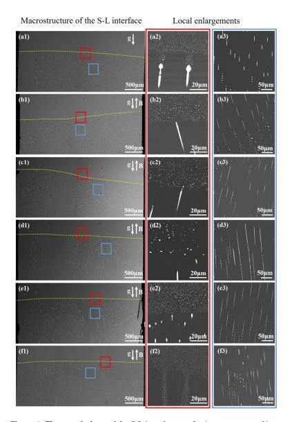
**Figure 2.** The morphology of the S-L interfaces and microstructures of ingots directionally solidified at a growth rate of 5  $\mu$ m/s under various MFDs. (a1–a3) 0 T; (b1–b3) 0.1 T; (c1–c3) 0.5 T; (d1–d3) 1 T; (e1–e3) 3 T; (f1–f3) 5 T. The yellow dotted lines are used to show the S-L interfaces.
