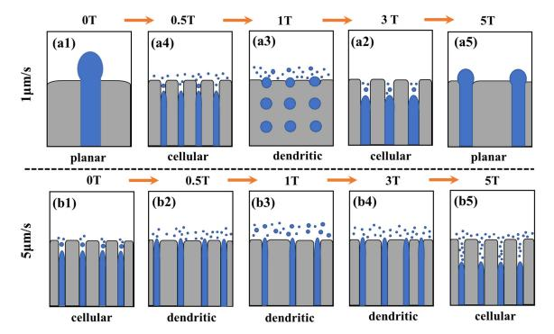
**Figure 5.** Schematic diagrams of the morphological evolution of the S-L interface in the ingots directionally solidified at growth rates of 1  $\mu$ m/s and 5  $\mu$ m/s, respectively, under various MFDs. (a1–a5) 1  $\mu$ m/s; (b1–b5) 5  $\mu$ m/s. The Bi-rich phases are colored in blue, and the Zn- rich matrixes are colored in grey.
