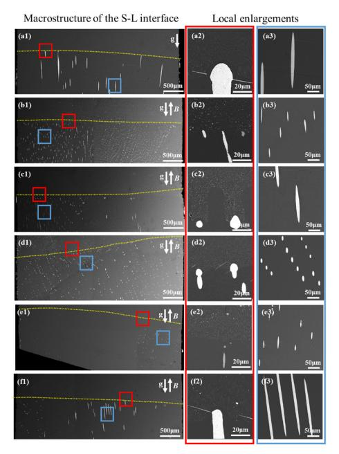
**Figure 1.** The morphology of the S-L interfaces and microstructures of ingots directionally solidified at a growth rate of 1  $\mu$ m/s under various MFDs. (a1–a3) 0 T; (b1–b3) 0.1 T; (c1–c3) 0.5 T; (d1–d3) 1 T; (e1–e3) 3 T, (f1–f3) 5 T. The yellow dotted lines are used to show the S-L interfaces.
