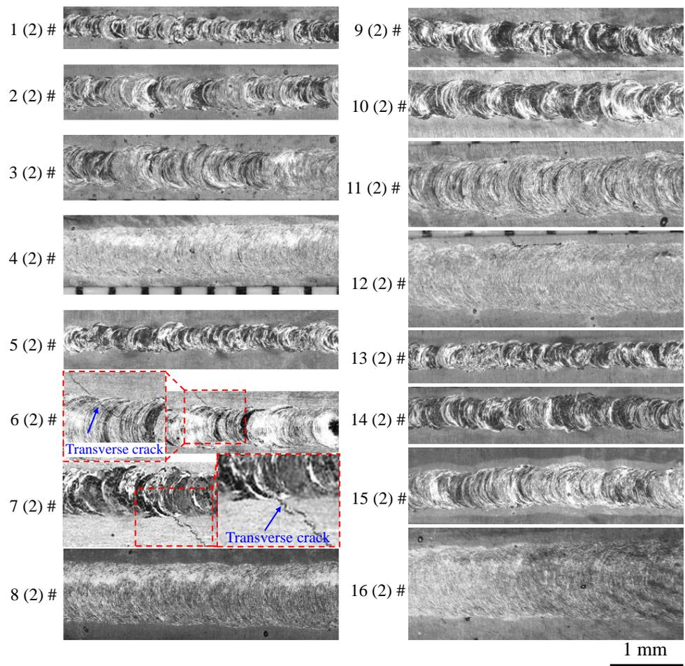
**Figure 6.** Macroscopic morphologies of the upper surface of the Mo–Re welding joints with a thickness of 2 mm.
