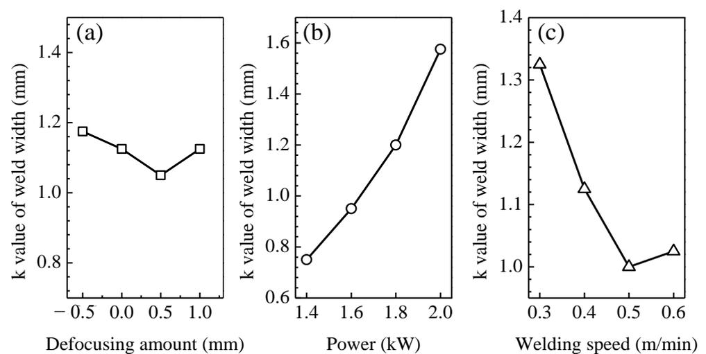
Figure 4. Relationships of (a) the defocusing amount, (b) power, and (c) welding speed with the weld width of Mo–Re joints with a thickness of 2 mm.
