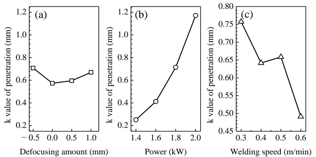
**Figure 3.** Relationships between (a) the defocusing amount, (b) power, and (c) welding speed with the penetration of the laser-welded joints of Mo–Re sheets with a thickness of 2 mm.
