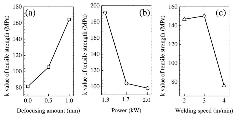
Figure 8. The relationships of (a) the defocusing amount, (b) power, and (c) welding speed with the maximum tensile strengths of the Mo–Re joints with a thickness of 0.5 mm.
