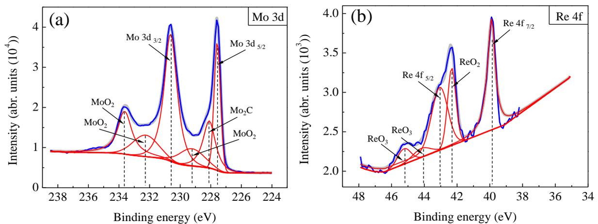
**Figure 13.** XPS results of Mo and Re elements: peak-fitting results of (a) Mo 3d and (b) Re 4f. The red curve indicates the spectrum of the phase used for the fitting, the blue curve indicates the fitted Mo3d spectrum and the gray curve indicates the original Mo3d spectrum.
