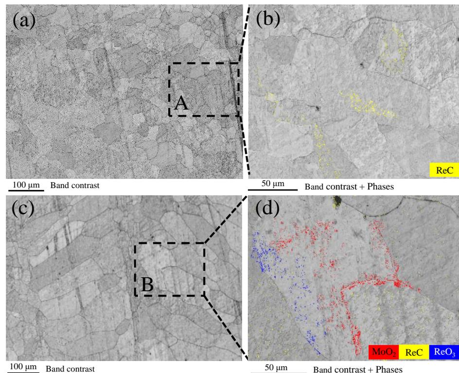
**Figure 14.** EBSD results in the BM and FZ of the Mo–Re alloy: (a) the band-contrast image of the BM; (b) the phase-distribution image of the A zone in the BM; (c) the band-contrast image of the FZ; (d) the phase-distribution image of the B zone in the FZ.
