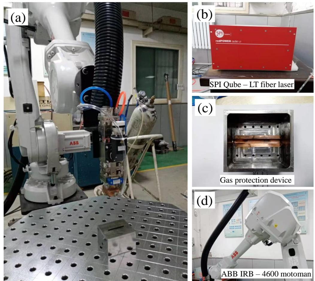
**Figure 2.** (a) The single-mode fiber laser welding system; (b) SPI fiber laser; (c) gas protection device; (d) ABB motorman.
