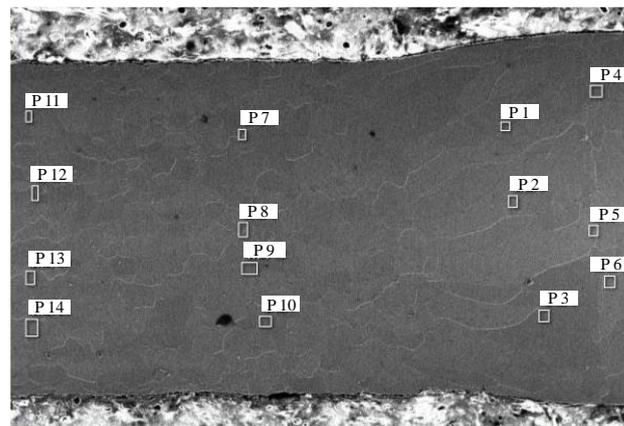
**Figure 12.** The measurement positions of the EDS point analysis on the cross section of the joint welded according to parameter (7 (0.5) #), P1–P14 indicates the sequence of EDS measurement positions and the white box indicates the EDS measurement position.
