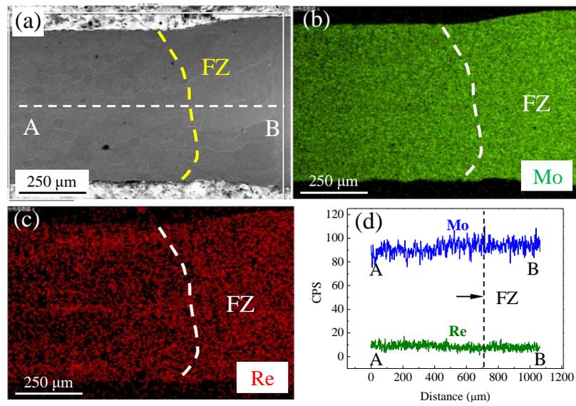
**Figure 11.** Result of EDS on the cross section of the joint welded using parameters 7 (0.5) #; (a) SEM image of the cross section; (b) the result of EDS area analysis of Mo; (c) the result of EDS area analysis of Re; (d) the result of EDS line scanning of Mo and Re along line AB in (a).
