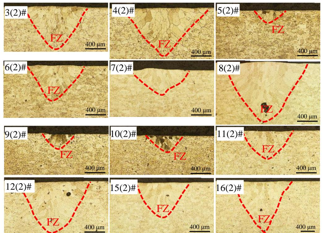
**Figure 5.** The metallographs of the cross sections of the Mo–Re joints with a thickness of 2 mm, obtained through a three-factor and four-level orthogonal test.
