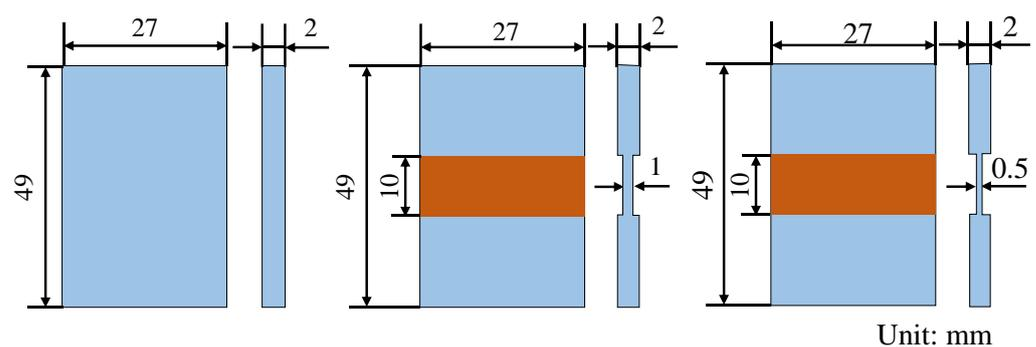
**Figure 1.** The specific dimensions of Mo–5Re sheets with thicknesses of 2 mm, 1 mm, and 0.5 mm.
