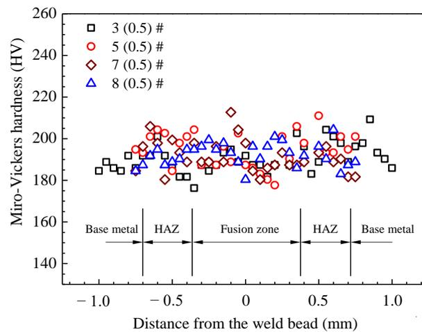
Figure 9. The hardness distribution of cross sections of the Mo–Re joints with a thickness of 0.5 mm.
