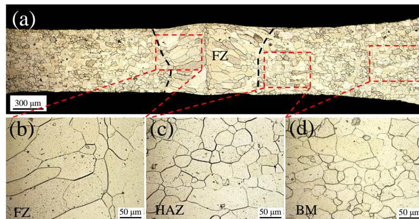
**Figure 10.** (a) Metallographic picture of the cross section of the joint welded using parameters 7 (0.5) #; (b–d) Magnified pictures of the FZ, HAZ, and BM, respectively.
