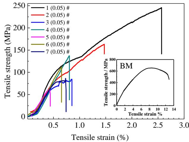
Figure 7. The stress–displacement curves of the Mo–Re welded joints with a thickness of 0.5 mm.
