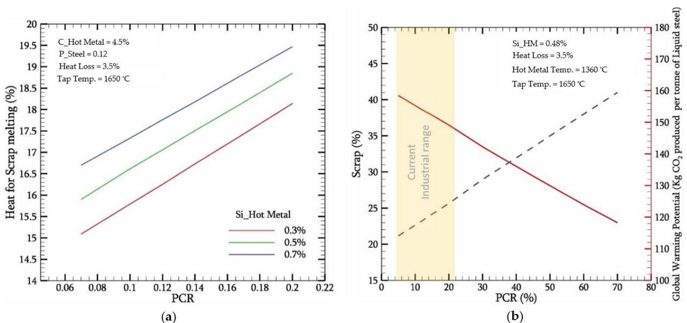
**Figure 8.** (a) Influence of PCR and Si in hot metal (%) on Heat of scrap melting (b) Effect of PCR (%) on scrap percentage and global warming potential.
