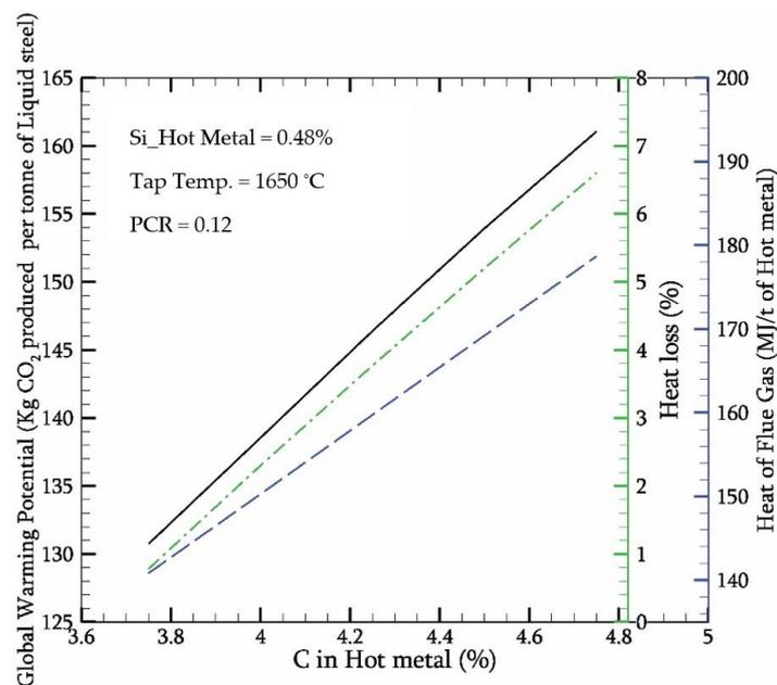
Figure 2. Effect of C in hot metal on GWP, heat loss, and heat of flue gas.
