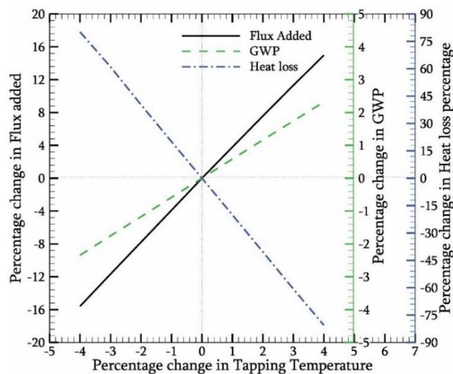
**Figure 5.** Effect of change in temperature on flux added, change in GWP, and change in heat loss percentage.
