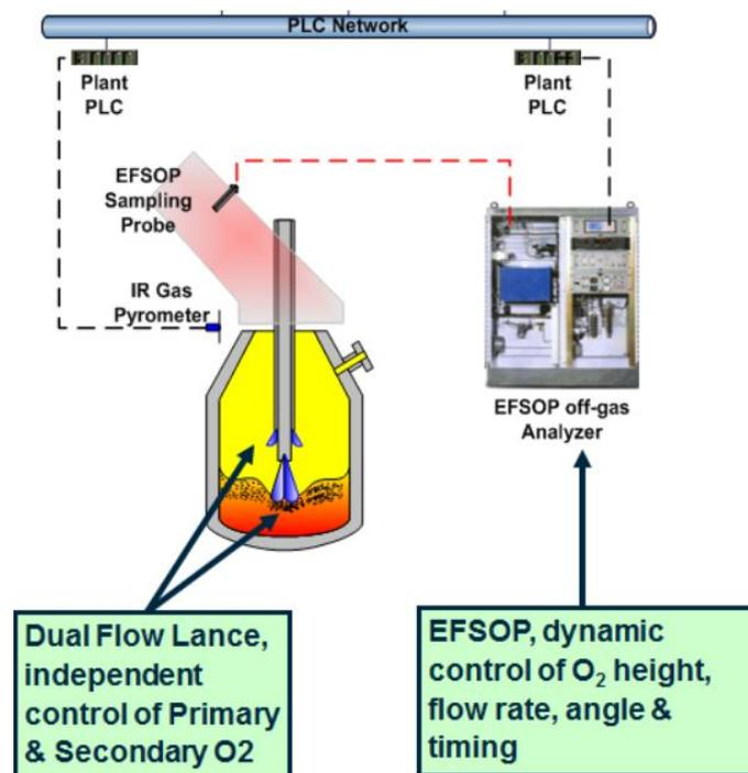
Figure 9. iBOF optimized post-combustion module, adapted from [48].
