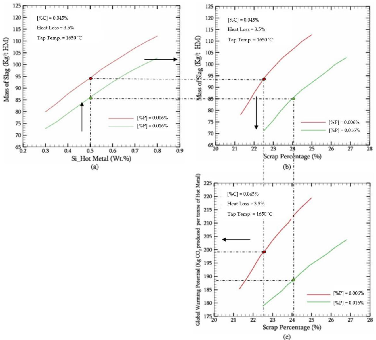
**Figure 6.** Nomogram from static balance model for top blow bottom stir technology with tap temperature of 1650 °C and assumed heat loss of 3.5%. (a) slag mass increase due to Si in Hot metal; (b) extra scrap due to additional heat; (c) additional amount of CO<sub>2</sub>.
