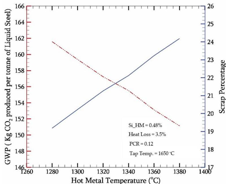
**Figure 7.** Effect of hot metal temperature on GWP of the process for a given PCR = 0.12, tapping temperature, silicon level, and heat loss.
