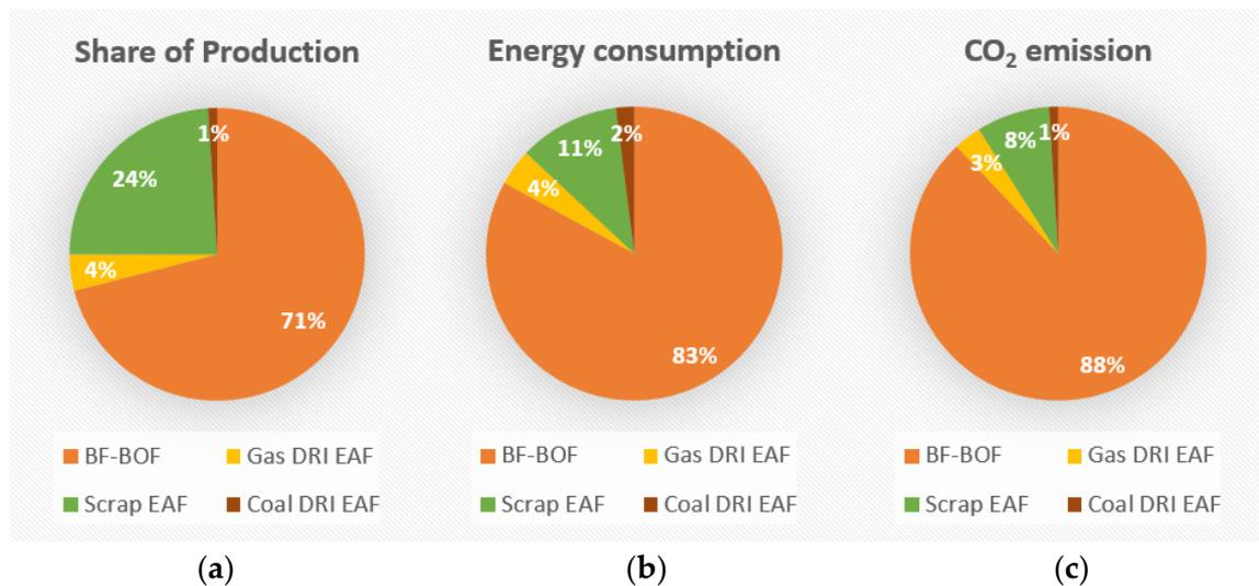
**Figure 1.** Share of worldwide (a) production, (b) energy consumption, and (c) CO<sub>2</sub> emission percentage via different steelmaking processes. Data from [2].
