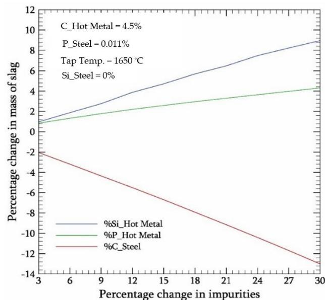
**Figure 3.** Sensitivity of impurities on mass of slag required for the process.
