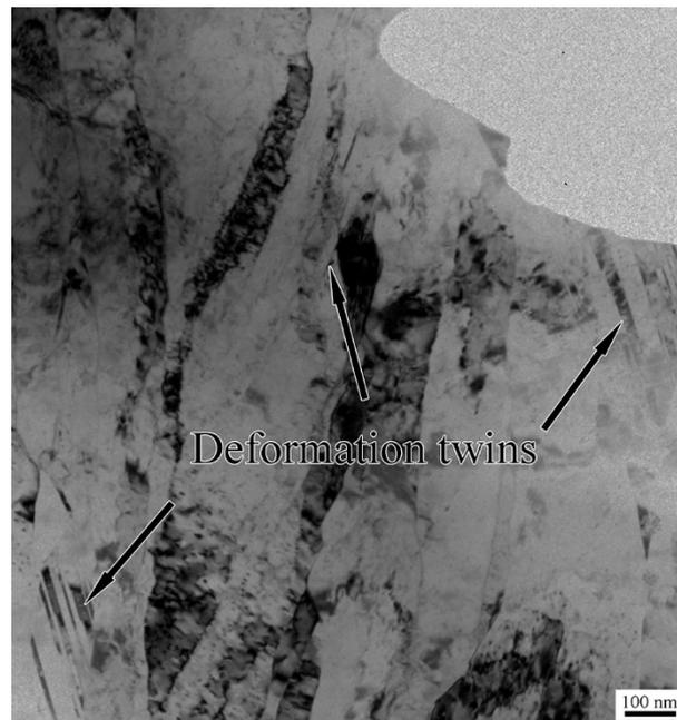
**Figure 5.** A high-magnification, longitudinal cross-section TEM observation of the aged Cu-0.4Cr-0.4Hf-S2.
