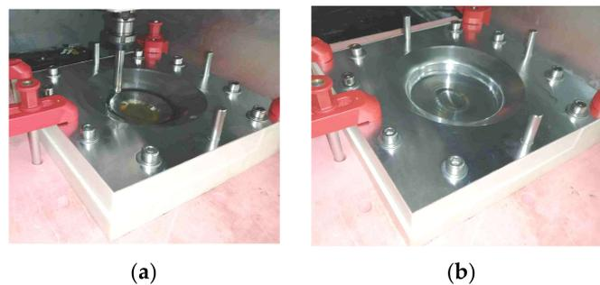
**Figure 29.** The proposed forming method: (a) the second-stage forming process; (b) the part formed by the second-stage forming.
