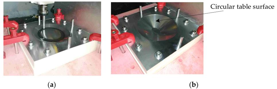
**Figure 28.** The proposed forming method: (a) the first-stage forming process; (b) the part formed by the first-stage forming.
