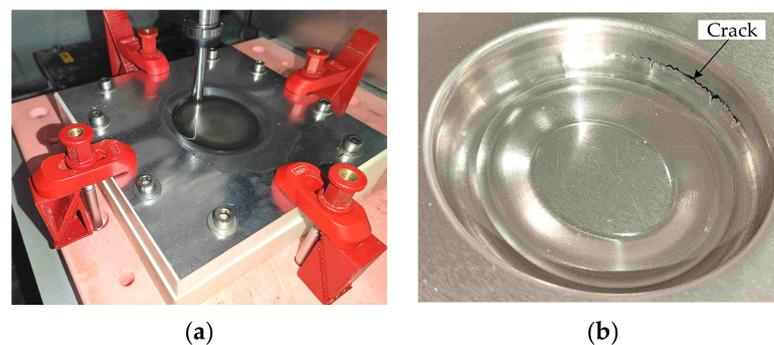
**Figure 27.** The traditional multistage forming: (a) the forming process; (b) the experimental part.
