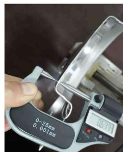
**Figure 33.** Thickness measurement.
