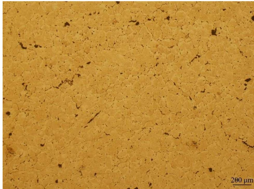
**Figure 6.** Microstructure of T6 heat-treated alloy.
