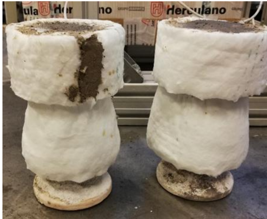
Figure 9. Thermal blanket applied around ceramic shell.
