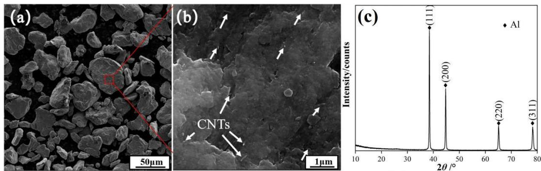
**Figure 3.** The microstructure and phase composition of milled CNTs/Al nanocomposites powders. (a,b) CNTs/Al; (c) XRD patterns of CNTs/Al.
