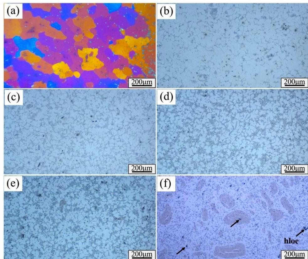
**Figure 5.** OM image. (a) Al-Cu-Mg-Si alloy; (b) 0.5 wt% CNTs/Al-Cu-Mg-Si composites; (c) 1.0 wt% CNTs/Al-Cu-Mg-Si composites; (d) 1.5 wt% CNTs/Al-Cu-Mg-Si composites; (e) 2.0 wt% CNTs/Al-Cu-Mg-Si composites; (f) 3.0 wt% CNTs/Al-Cu-Mg-Si composites.
