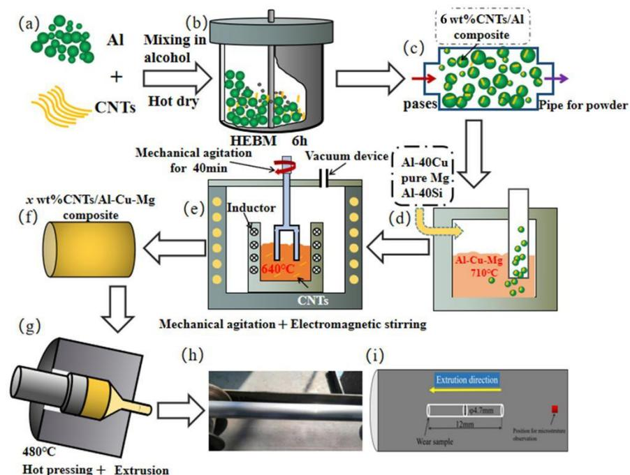
**Figure 1.** (a–i) Schematic diagram of preparation route for  $x\%$  CNTs/Al-Cu-Mg-Si composites and semi-solid stir casting.
