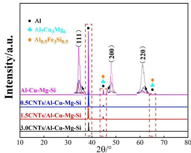
Figure 4. XRD patterns of CNTs/Al-Cu-Mg-Si composites.
