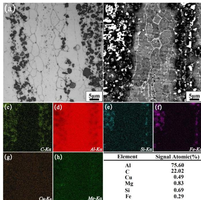
**Figure 6.** Microstructure of as hot-extrusion 1.5 wt% CNT/Al-Cu-Mg-Si composite. (a) OM image of macrostructure, (b–h) SEM back-scattered electron image (Determine the distribution of C, Al, Si, Fe, Cu, Mg by scanning the EDS surface).
