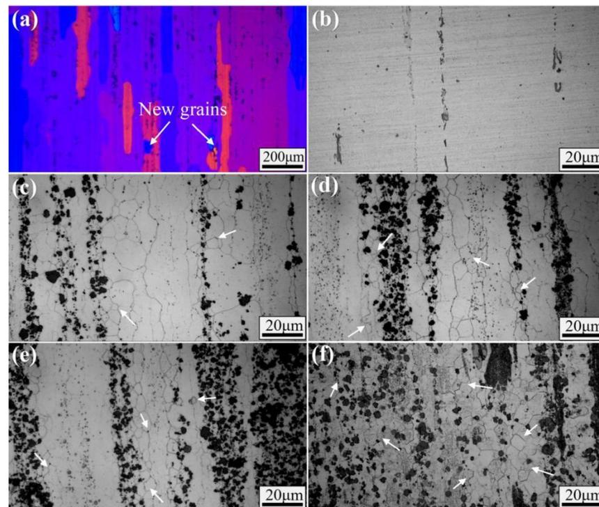
**Figure 8.** Microstructures along the extrusion direction. (a) Al-Cu-Mg-Si alloy; (b) 0.5 wt% CNTs/Al-Cu-Mg-Si composites; (c) 1.0 wt % CNTs/Al-Cu-Mg-Si composites; (d) 1.5 wt % CNTs/Al-Cu-Mg-Si composites; (e) 2.0 wt % CNTs/Al-Cu-Mg-Si composites; (f) 3.0 wt % CNTs/Al-Cu-Mg-Si composites.
