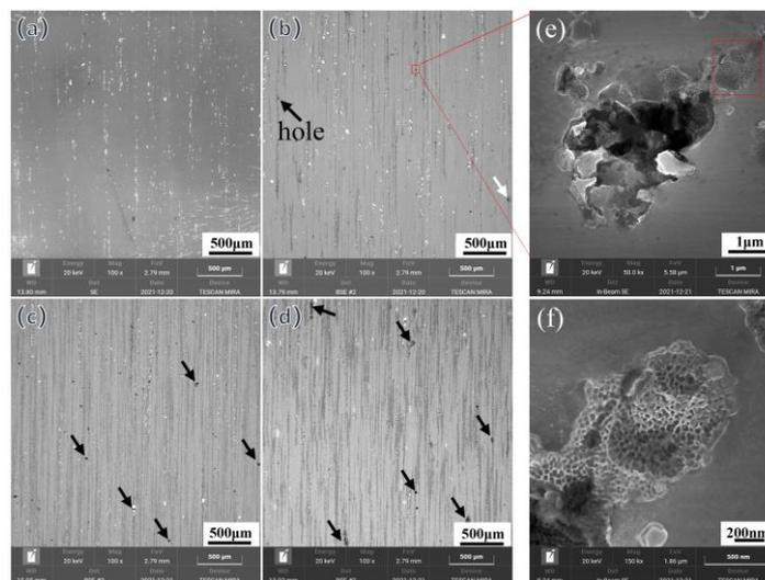
**Figure 7.** SEM image of  $x\%$  CNTs/Al-Cu-Mg-Si composites. (a) Al-Cu-Mg-Si alloy; (b) 1.5 wt% CNTs/Al-Cu-Mg-Si composites; (c) 2.0 wt% CNTs/Al-Cu-Mg-Si composites; (d) 3.0 wt% CNTs/Al-Cu-Mg-Si composites; (e,f) High magnification morphology at holes.
