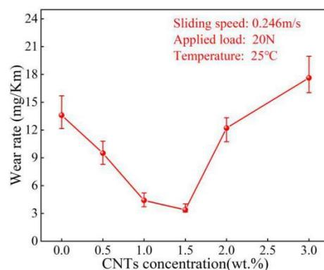
**Figure 11.** Wear rate versus CNT wt%.
