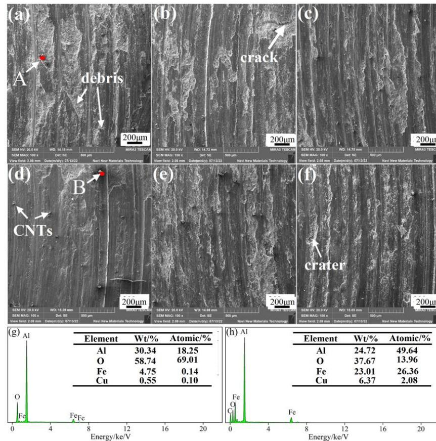
**Figure 15.** SEM micrographs of representative worn surfaces of  $x\%$  CNTs / Al-Cu-Mg-Si under 200 °C: (a) 0 wt%, (b) 0.5 wt%, (c) 1.0 wt%, (d) 1.5 wt%, (e) 2.0 wt%, (f) 3.0 wt%. (g) EDS result of point A, (h) EDS result of point B.
