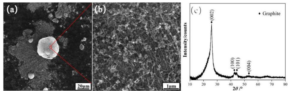
**Figure 2.** The microstructure and phase composition of raw powders. (a,b) CNTs; (c) XRD patterns of CNTs.
