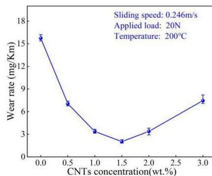
**Figure 14.** Wear rate of the  $x\%$  CNTs / Al-Cu-Mg-Si composites under 200 °C.
