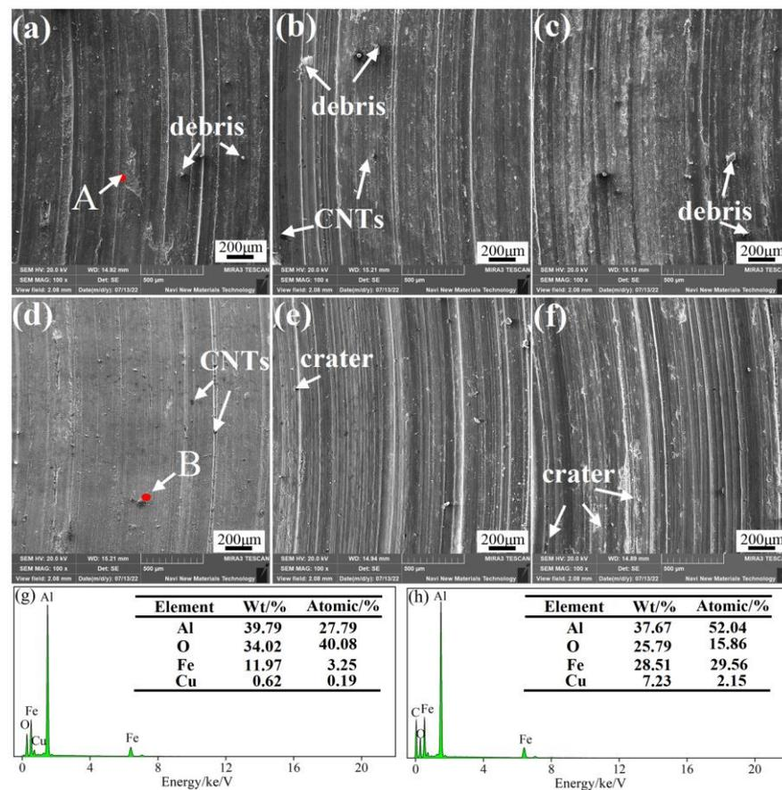
**Figure 12.** SEM micrographs and EDS of representative worn surfaces of  $x\%$  CNTs/Al-Cu-Mg-Si: (a) 0 wt%, (b) 0.5 wt%, (c) 1.0 wt%, (d) 1.5 wt%, (e) 2.0 wt%, (f) 3.0 wt%, (g) EDS result of point A, (h) EDS result of point B.
