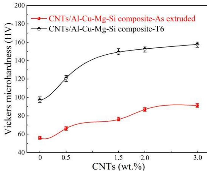
**Figure 9.** Results from the microhardness test of CNTs/Al-Cu-Mg-Si composites.
