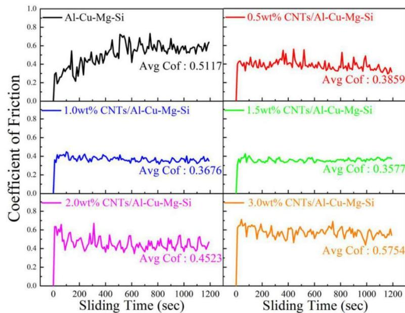
**Figure 10.** Plot of the coefficient of friction as a function of sliding time for:  $x$  wt%CNTs / Al-Cu-Mg-Si composites at 20 °C.
