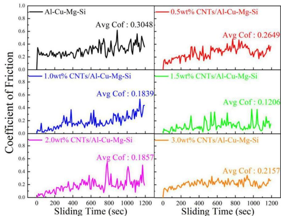
**Figure 13.** Plot of the coefficient of friction as a function of sliding time for  $x\%$  CNTs / Al-Cu-Mg-Si composites under 200 °C.
