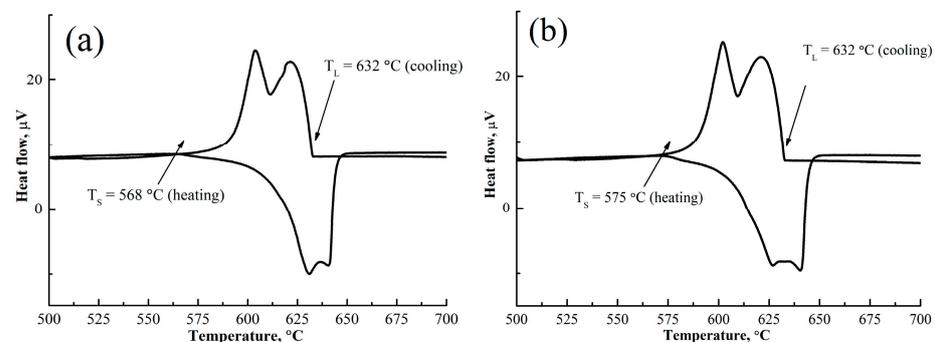
**Figure 3.** DSC curves of the (a) AlCuYbMg and (b) AlCuGdMg alloys.
