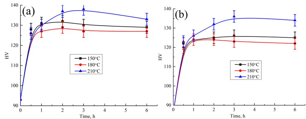
**Figure 6.** Aging curves of the (a) AlCuYbMg and (b) AlCuGdMg alloys.
