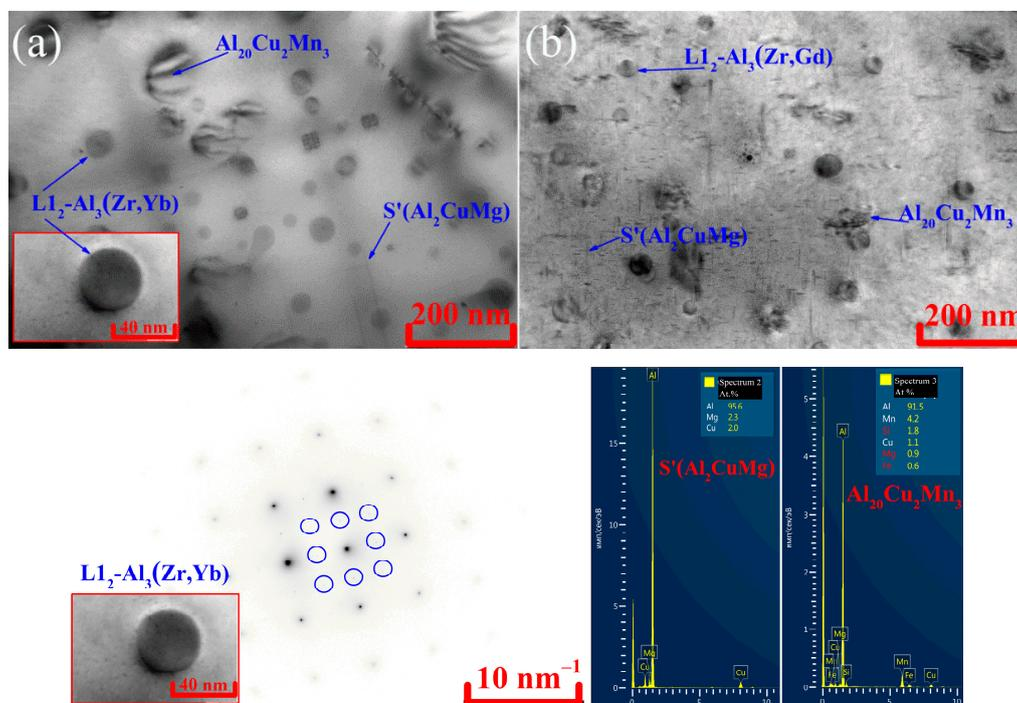
**Figure 5.** Microstructures of the (a) AlCuYbMg and (b) AlCuGdMg alloys after 3 h of solution treatment at (a) 555 °C and (b) 565 °C, quenching and aging at 210 °C for 3 h, and FFT pattern of  $L1_2$ - $Al_3$ (Zr,Yb), and EDX spectrum from  $S'$  and  $Al_{20}Cu_2Mn_3$  phases (TEM).
