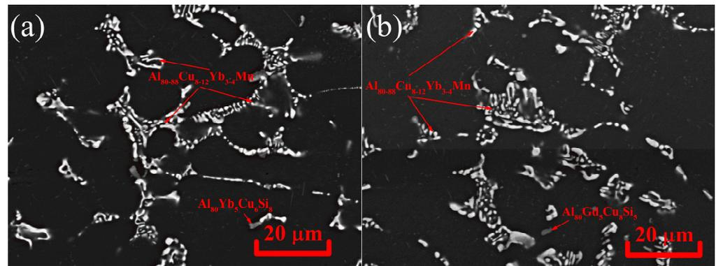
**Figure 4.** Microstructures of the (a) AlCuYbMg and (b) AlCuGdMg alloys after 3 h of solution treatment at (a) 555 °C and (b) 565 °C (SEM-BSE).
