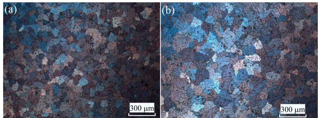
**Figure 1.** As-cast grain structures of the (a) AlCuYbMg and (b) AlCuGdMg alloys (OM).
