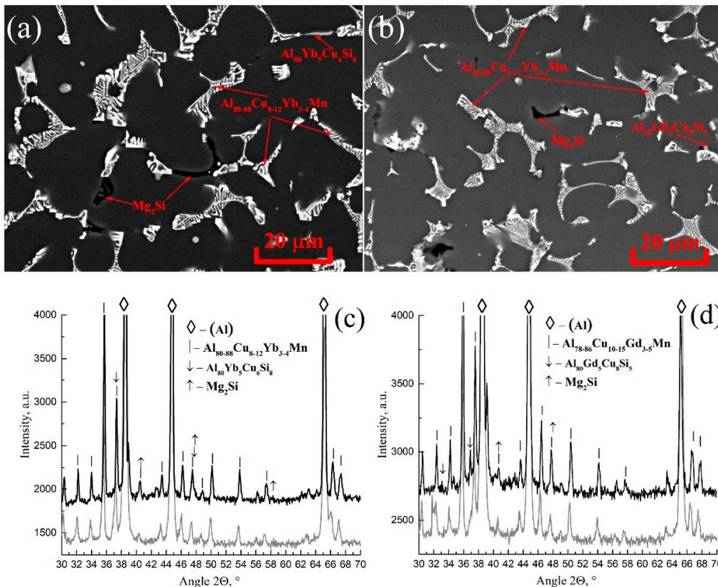
**Figure 2.** As-cast microstructure and phase composition of the (a,c) AlCuYbMg and (b,d) AlCuGdMg alloys ((a,b)—SEM-BSE phase composition, (c,d)—XRD (grey lines—Mg-,Si- and Fe-free alloys)).
