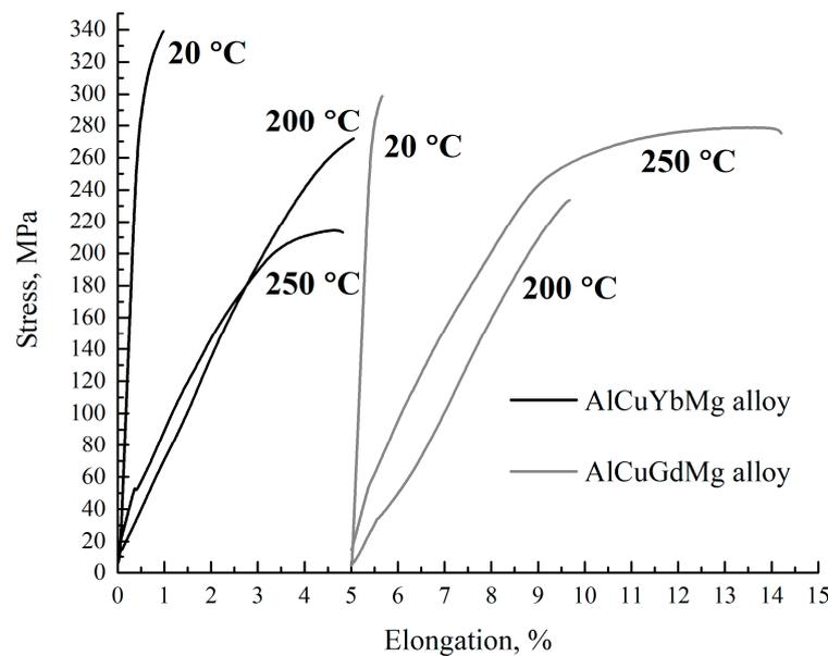
Figure 7. Typical tensile curves of the AlCuYbMg and AlCuGdMg alloys at different temperatures.
