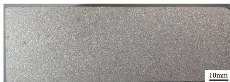
**Figure 3.** Macrostructure of as-cast AA6063.
