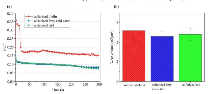
**Figure 4.** (a) Friction coefficients and (b) wear volume when lubricated by sulfur additives at 150 °C (F = 100 N, f = 20 Hz, L = 2 mm).
