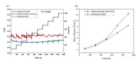
**Figure 6.** (a) Friction coefficient vs. time during a load slope test from 100 N to 1000 N and (b) wear volume under different loads (f = 20 Hz, L = 2 mm, t = 25 °C).
