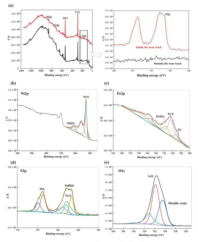
formed, playing a role in lubrication. The physical adsorptive film and the tribochemical film together enhance the friction-reducing and anti-wear performances of the lubricants.
