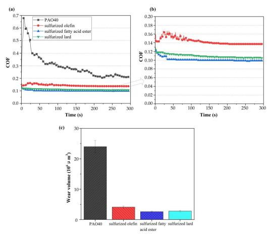
**Figure 2.** (a) Friction coefficients with (b) enlarged view, and (c) wear volume of the discs lubricated by different lubricants (F = 100 N, f = 20 Hz, L = 2 mm).
