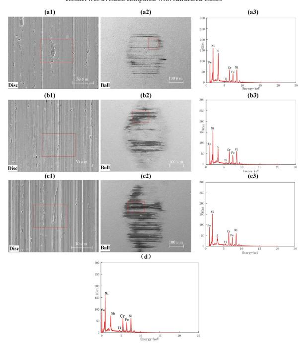
**Figure 3.** SEM morphology of the tracks on Inconel 718 and tungsten carbide ball lubricated by (a1,a2) sulfurized olefin, (b1,b2) sulfurized fatty acid ester, and (c1,c2) sulfurized lard; (a3,b3,c3) EDS spectrum of the red box in (a1,b1,c1); (d) EDS spectrum of the red box in (a2).
