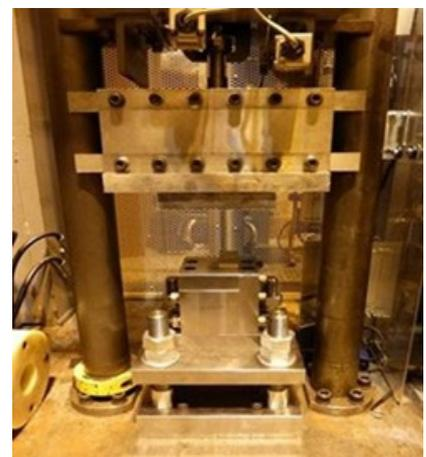
Figure 2. Impact joining device: (a) Cross-sectional schematic; (b) General view and drop weight.
