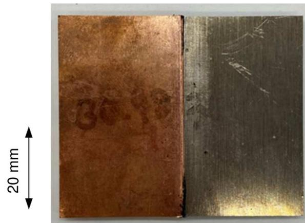
**Figure 13.** Joined specimen using shaved face (left: C1100, right: A6061, shaving allowance: C1100 1.0 mm, A6061 0.9 mm, overlap length: 0.1 mm).
