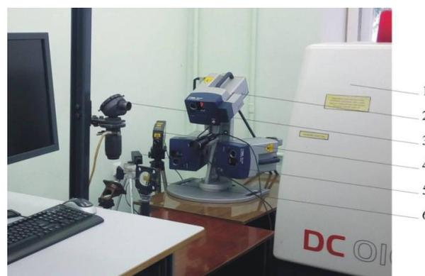
**Figure 8.** Photo of the experimental setup for studying vibration characteristics of objects during the formation of laser-induced nanopores: 1—diffusion-cooled and radio-frequency excited  $\text{CO}_2$ -laser; 2—three-axis scanning laser vibrometer; 3—optical system; 4—two-coordinate measuring instrument; 5—non-contact thermometer; 6—sample of brass L62 [74].
