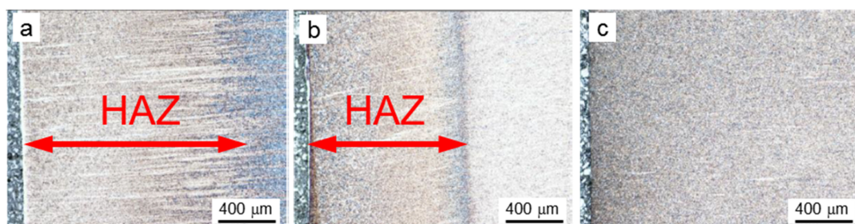
Figure 1. Optical microscopy images of heat affected zone in Steel H cut with (a) oxy-fuel, (b) plasma, and (c) water-jet.
