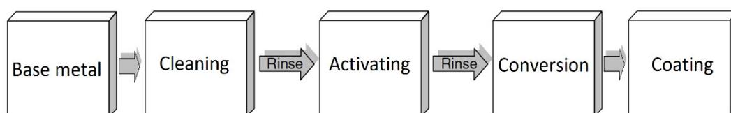
**Figure 22.** Standard initial steps of a process chain of handling magnesium surfaces (conversion coating in this example).
