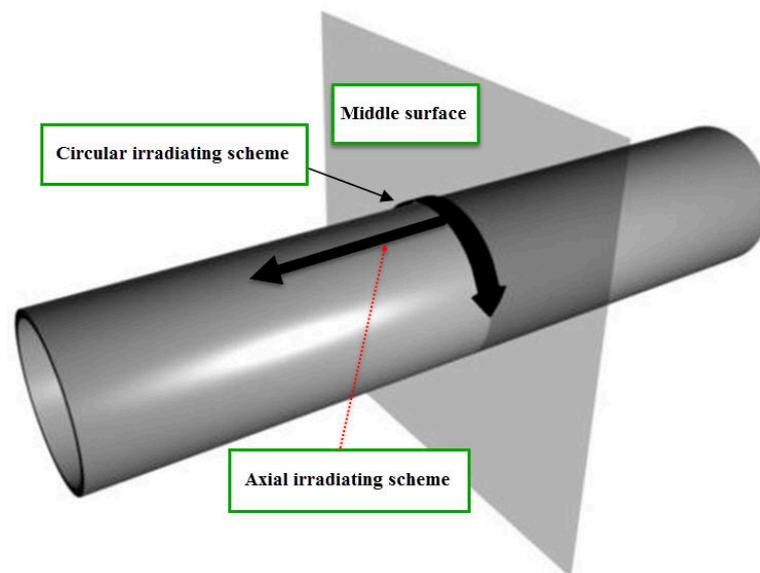
**Figure 3.** The schematics of the circular irradiating scheme (CIS) and axial irradiating scheme (AIS).
