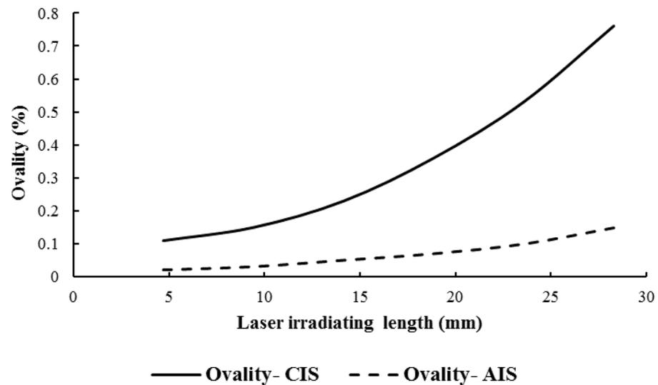
**Figure 6.** The effect of irradiating schemes on the ovality percentage of laser-bent tubes.
