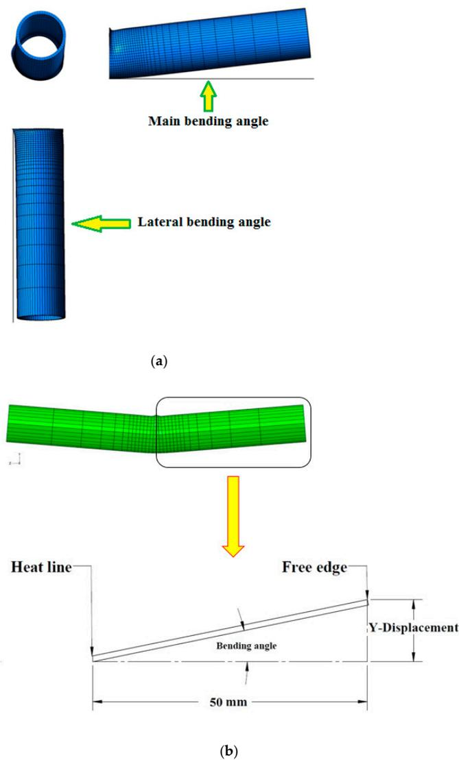
**Figure 2.** (a) Schematic views of main and lateral bending angles, (b) Schematic view of the main bending angle relevant to Y-displacement for a laser-bent tube.
