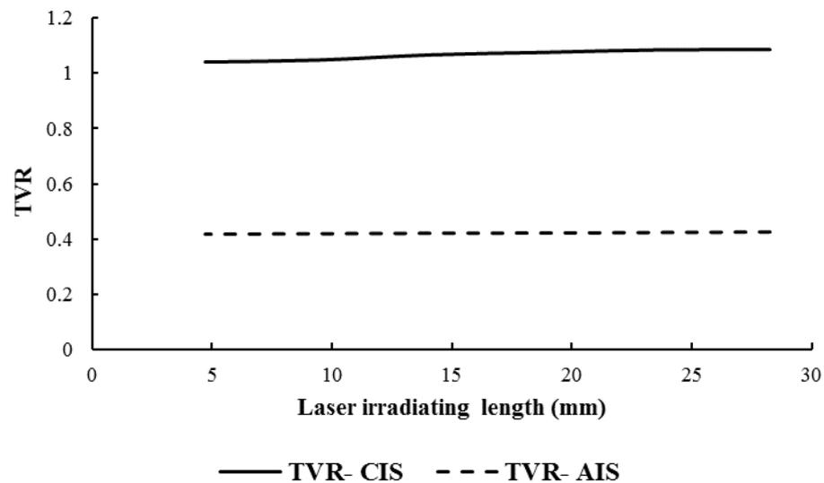
**Figure 7.** The effects of irradiating scheme on thickness variation ratio (TVR) of the laser-bent tubes.
