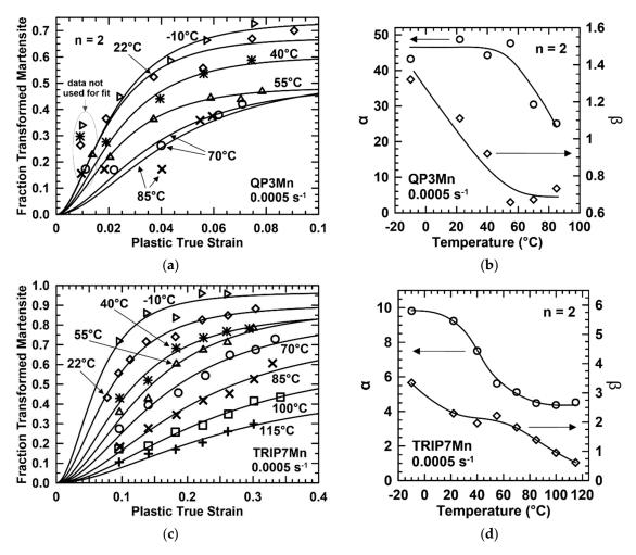
**Figure 5.** Fraction of transformed martensite versus plastic strain at various test temperatures (0.0005 s<sup>-1</sup> strain rate) for (**a**) QP3Mn and (**c**) TRIP7Mn. The points are experimental data, and the curves are the Olson–Cohen model fits. For QP3Mn, data at 2% and greater strain were used for model fits. Olson–Cohen model parameters *α* and *β* versus temperature with *n* equal to 2 for (**b**) QP3Mn and (**d**) TRIP7Mn.
