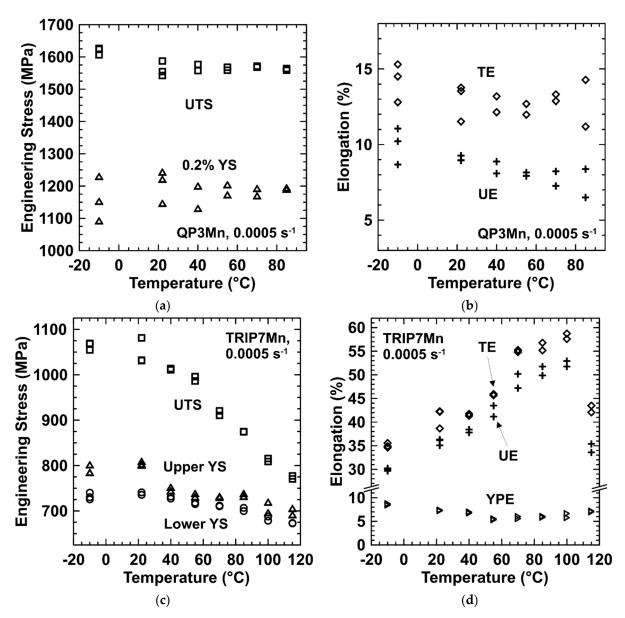
**Figure 6.** Tensile mechanical properties versus temperature from replicate tests at  $0.0005 \, \text{s}^{-1}$ . (a) QP3Mn 0.2% YS and UTS; (b) QP3Mn UE and TE; (c) TRIP7Mn lower YS, upper YS, and UTS; and (d) TRIP7Mn YPE, UE, and TE.
