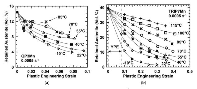
**Figure 4.** Austenite volume fraction versus plastic strain from tests at  $0.0005 \, \mathrm{s}^{-1}$  and various temperatures for (a) QP3Mn and (b) TRIP7Mn.
