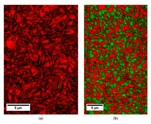
**Figure 2.** Combined EBSD phase map and image quality map showing the as-processed microstructures of (a) QP3Mn and (b) TRIP7Mn. Red indicates ferrite/martensite and green indicates austenite.
