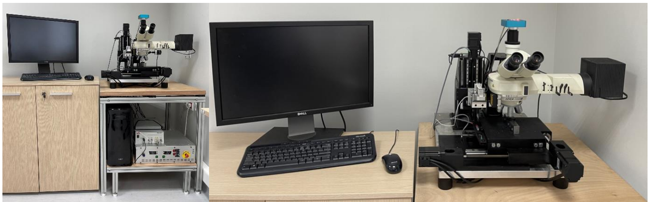
Figure 6. Nanoindentation test of nanocrystalline specimens according to ISO 14577.
