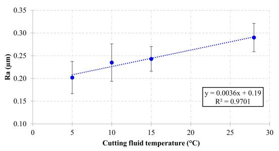
Figure 3. Surface roughness (Ra parameter) of the ground surface as a function of cutting fluid temperature.
