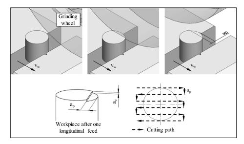
Figure 1. Sketch of the grinding operation used in the experimental trials.
