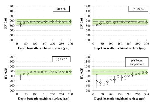
**Figure 5.** Microhardness as a function of depth beneath the machined surface after grinding with the cutting fluid applied at different temperatures: (**a**) 5 °C; (**b**) 10 °C; (**c**) 15 °C; and (**d**) room temperature.
