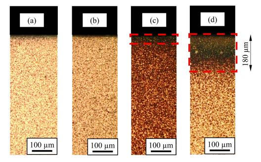
**Figure 6.** Microstructure beneath the machined surface after grinding with cutting fluid at different temperatures: (a)  $5 \degree C$ ; (b)  $10 \degree C$ ; (c)  $15 \degree C$ ; and (d) room temperature.
