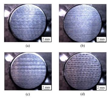
**Figure 4.** Images of the machined surface after grinding with cutting fluid at different temperatures: (a)  $5 \degree C$ ; (b)  $10 \degree C$ ; (c)  $15 \degree C$ ; and (d) room temperature.
