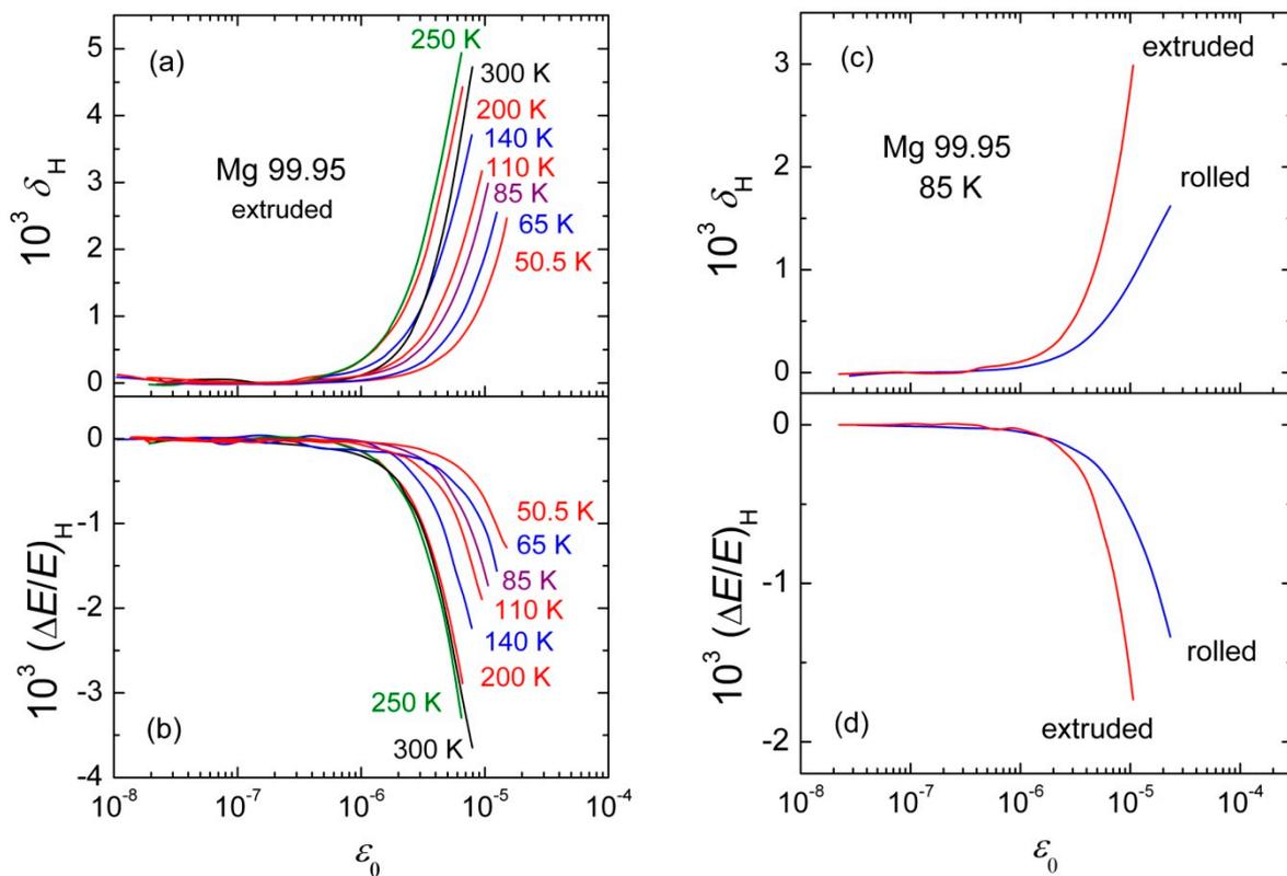
**Figure 6.** Effect of the temperature (a,b) and deformation mode (c,d) on the amplitude-dependent part of the decrement  $\delta_H$  and the modulus defect  $(\Delta E/E)_H$  in the extruded and rolled samples.
