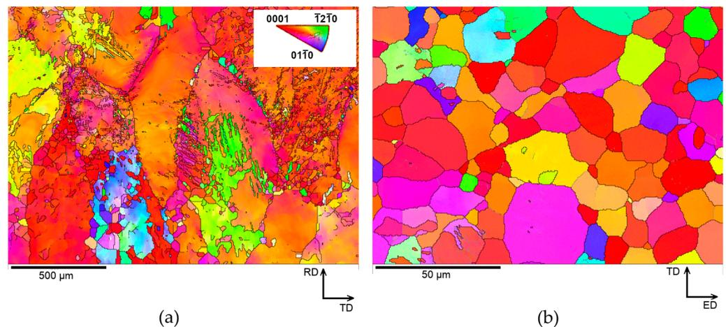
**Figure 2.** Electron backscattered diffraction (EBSD) maps for (a) rolled (inset—orientation color key) and (b) extruded Mg samples. The maps were collected from RD-TD plane or ED-TD plane in the case of rolling and extrusion, respectively.
