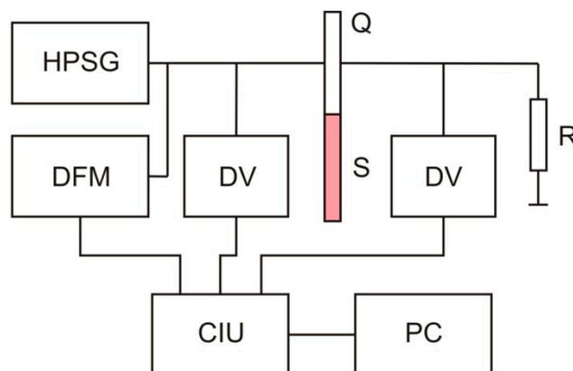
**Figure 5.** Block diagram of the experimental setup for measuring by the two-component composite vibrator techniques in the ultrasonic frequency range. HPSG is the high precision signal generator; DV are the digital voltmeters; DFM is the digital frequency meter; CIU is the control and interfaces unit; PC is a personal computer; Q is a piezoelectric quartz transducer; S is the sample under study.
