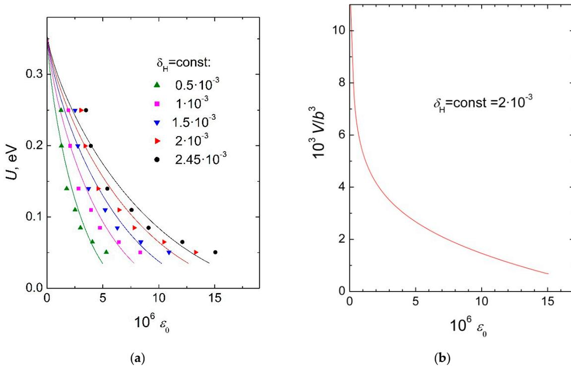
**Figure 8.** Dependences (a) of the activation energy  $U$  on amplitude  $\varepsilon_0$  for several sections  $\delta_H(T, \varepsilon_0) = \text{const}$  and (b) the activation volume  $V$  for the section  $\delta_H(T, \varepsilon_0) = 2 \times 10^{-3}$  for the extruded sample.
