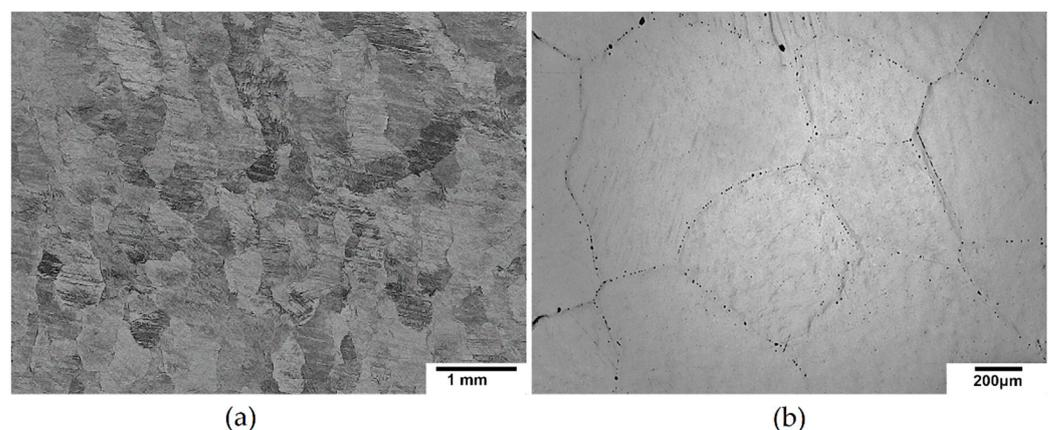
**Figure 1.** Light micrographs of initial as-cast material used (a) for rolling and (b) for extrusion.
