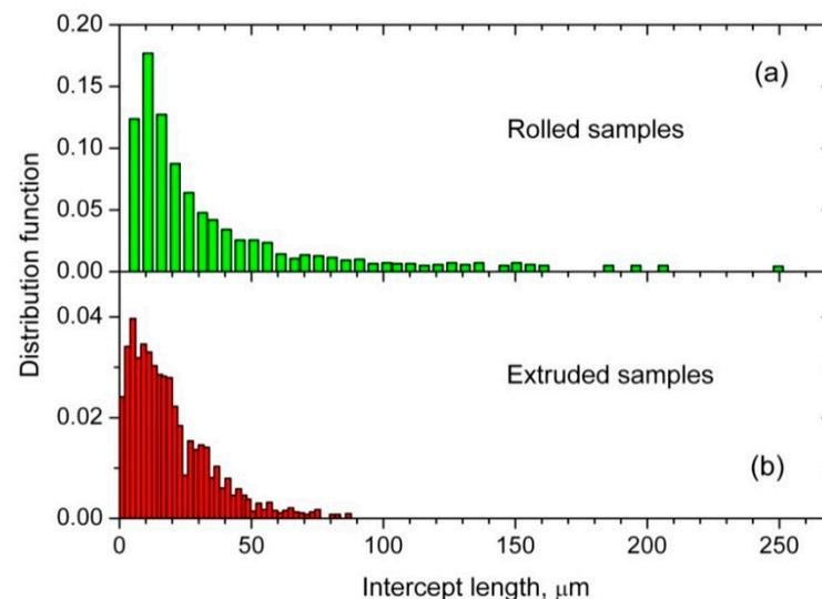
**Figure 3.** Distribution of grain sizes in (a) rolled and (b) extruded samples.
