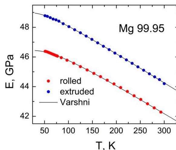
**Figure 9.** Temperature dependences of the dynamic Young's modulus of rolled and extruded Mg samples. Solid lines show the approximations made using Equation (8).
