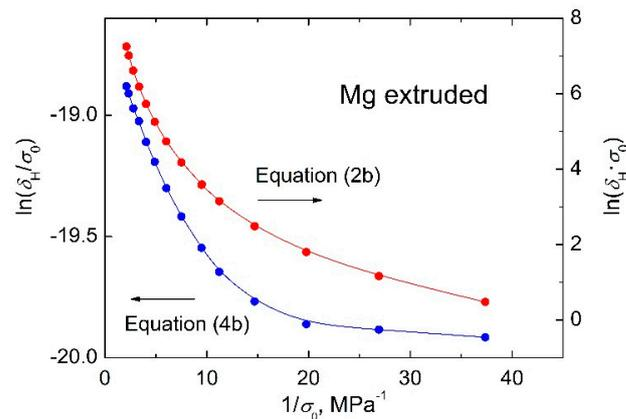
**Figure 7.** Failed attempts to linearize experimental data using Equation (2b) (right-hand axis) and Equation (4b) (left-hand axis). It can be seen that Equations (2b) and (4b) do not lead to a straightening of the experimental dependences in the coordinates proposed.
