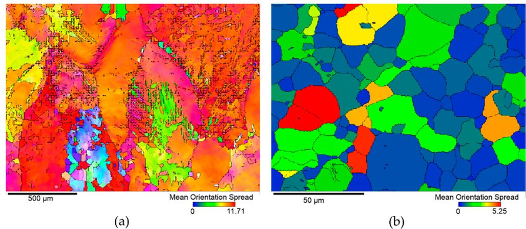
**Figure 10.** Grain orientation spread (GOS) maps of (a) rolled and (b) extruded sample.
