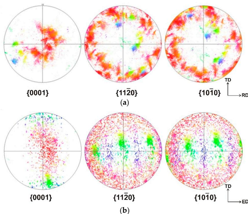
**Figure 4.** Pole figures of (a) rolled Mg samples (rolling direction RD, right; transverse direction TD, top; normal direction ND, projection plane) and (b) extruded Mg samples (extrusion direction ED, right; transverse direction TD, top; normal direction ND, projection plane).
