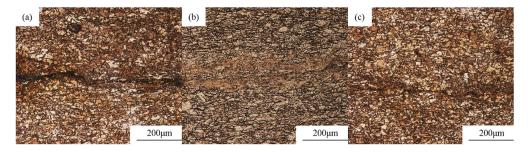
**Figure 7.** Metallographic diagram of the joints with different welding heat inputs: (**a**) 700 J; (**b**) 980 J; (**c**) 1260 J.
