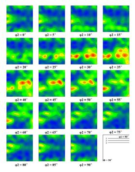
Figure 16. ODF diagram of a copper ultrasonic welding joint.
