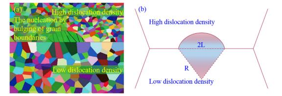
**Figure 19.** Schematic diagram of DDRXODF nucleation: (**a**) Nucleation by bulging of grain boundaries; (**b**) nucleation model [18,30].
