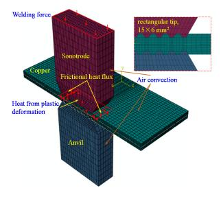
Figure 4. Finite element model of Cu-ETP ultrasonic welding.
