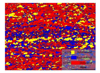
Figure 18. EBSD recrystallization fraction statistics graph of the welded joint.
