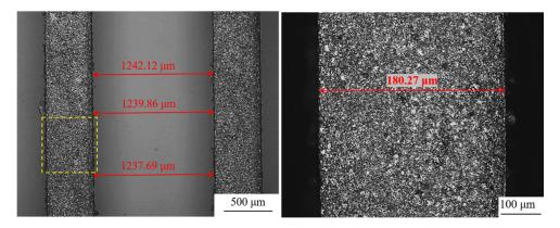
Figure 2. Straight groove shape and size of the micro-EDM.
