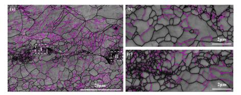
Figure 13. Grain boundary map of the Cu-ETP ultrasonic welded joint (a), grain boundary map in zone I (b) and II (c).
