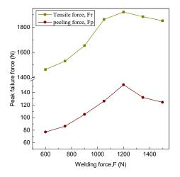
Figure 10. Tensile and peeling peak failure load with different welding forces.
