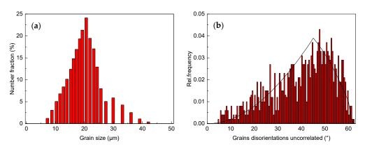
Figure 12. Statistical graph of the base metal grain size (a) and misorientation (b).
