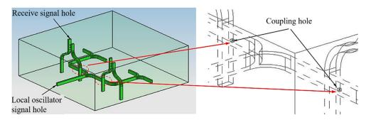
Figure 1. Schematic diagram of the 3D metal waveguide network.
