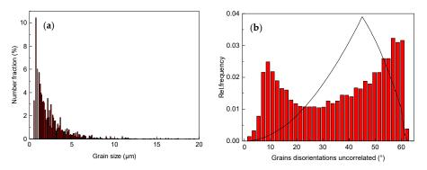
Figure 14. Statistical graph of the welded joint grain size (a) and misorientation (b).
