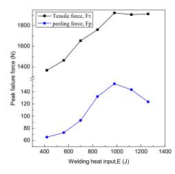
Figure 8. Tensile and peeling peak failure load with different welding heat inputs.
