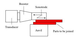
Figure 3. Scheme of metal ultrasonic welding.
