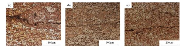
Figure 9. Metallographic diagram of the joints with different welding forces: (a) 600 N; (b) 1200 N; (c) 1400 N.
