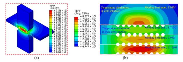
Figure 17. Temperature distribution at different welding heat inputs for the 3D plot (a) and xy plot (b).
