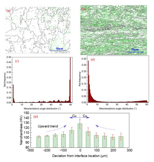
addition, these misorientations include not only the grain boundaries, but also the sub-grain boundaries inside the grains (Figure 12b).
