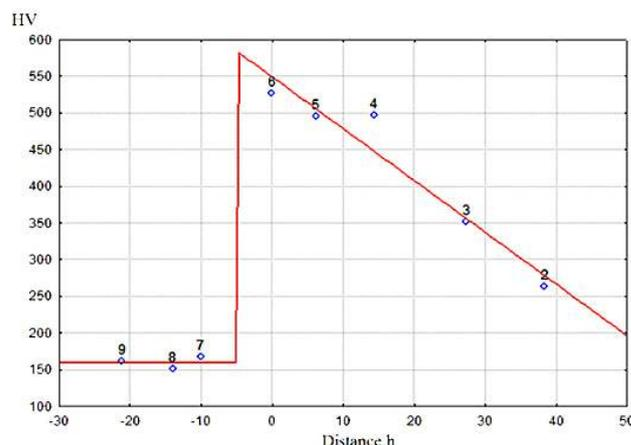
Figure 8. Piecewise approximation of microhardness distribution in the bimetal interface (SLM mode 2).
