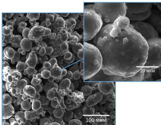
**Figure 1.** Scanning electron microscopy images of Al-Si10-Mg powder.
