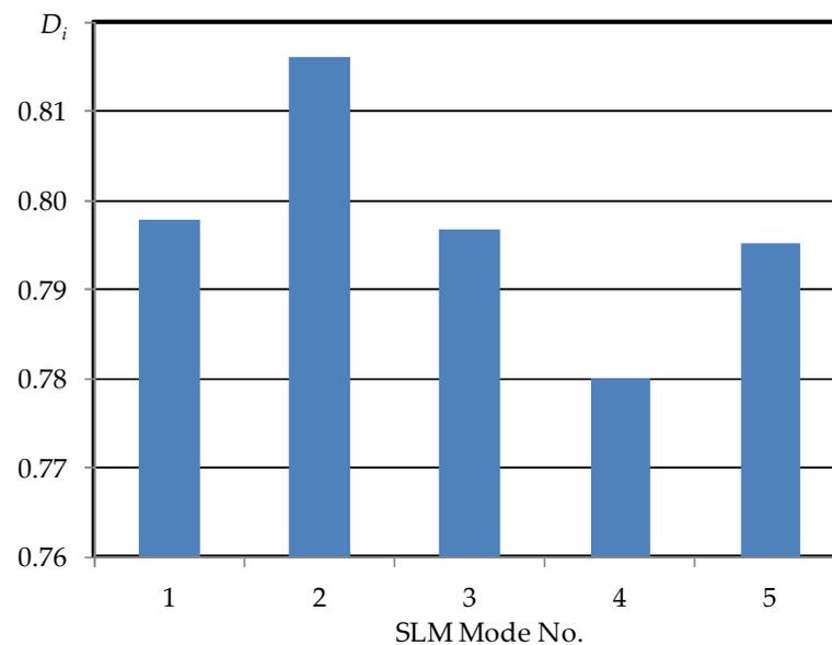
**Figure 10.** The generalized desirability function of quality indices for different SLM technological modes.
