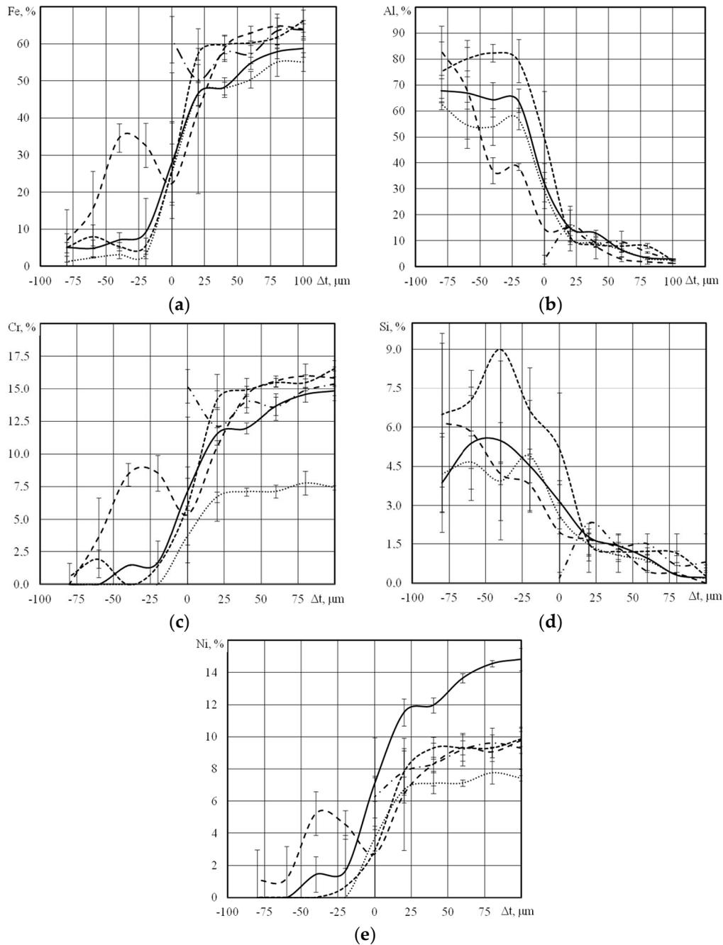
**Figure 5.** Distribution of chemical elements Fe (a), Al (b), Cr (c), Si (d) and Ni (e) at the bimetal interface zone: SLM mode 1; SLM mode 2; SLM mode 3; SLM mode 4; SLM mode 5.
