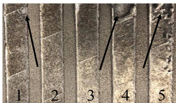
**Figure 3.** A general view of the sintered specimens: 1—SLM mode 1; 2—SLM mode 2; 3—SLM mode 3; 4—SLM mode 4; 5—SLM mode 5; arrows—defects.
