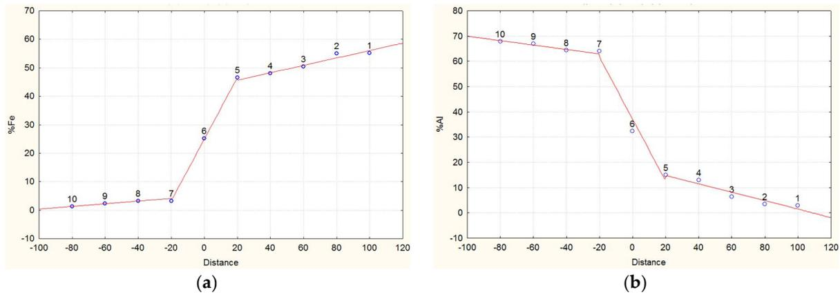
**Figure 7.** Piecewise linear approximation of Fe (a) and Al (b) content in the bimetal interface (SLM mode 2).
