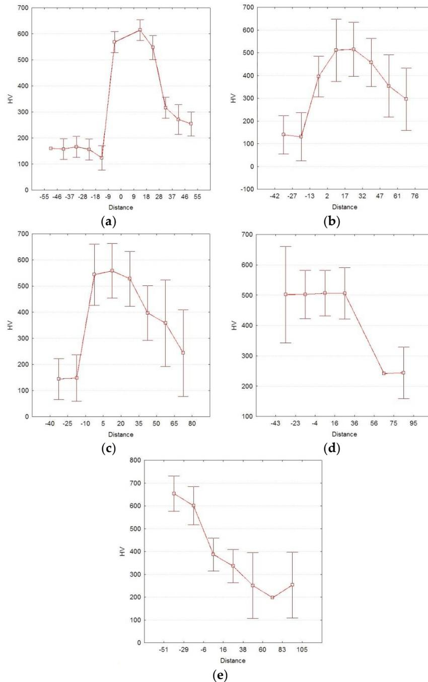
**Figure 6.** Distribution of hardness at the bimetal interface zone: (a) SLM scanning mode 1; (b) SLM scanning mode 2; (c) SLM scanning mode 3; (d) SLM scanning mode 4; (e) SLM scanning mode 5.
