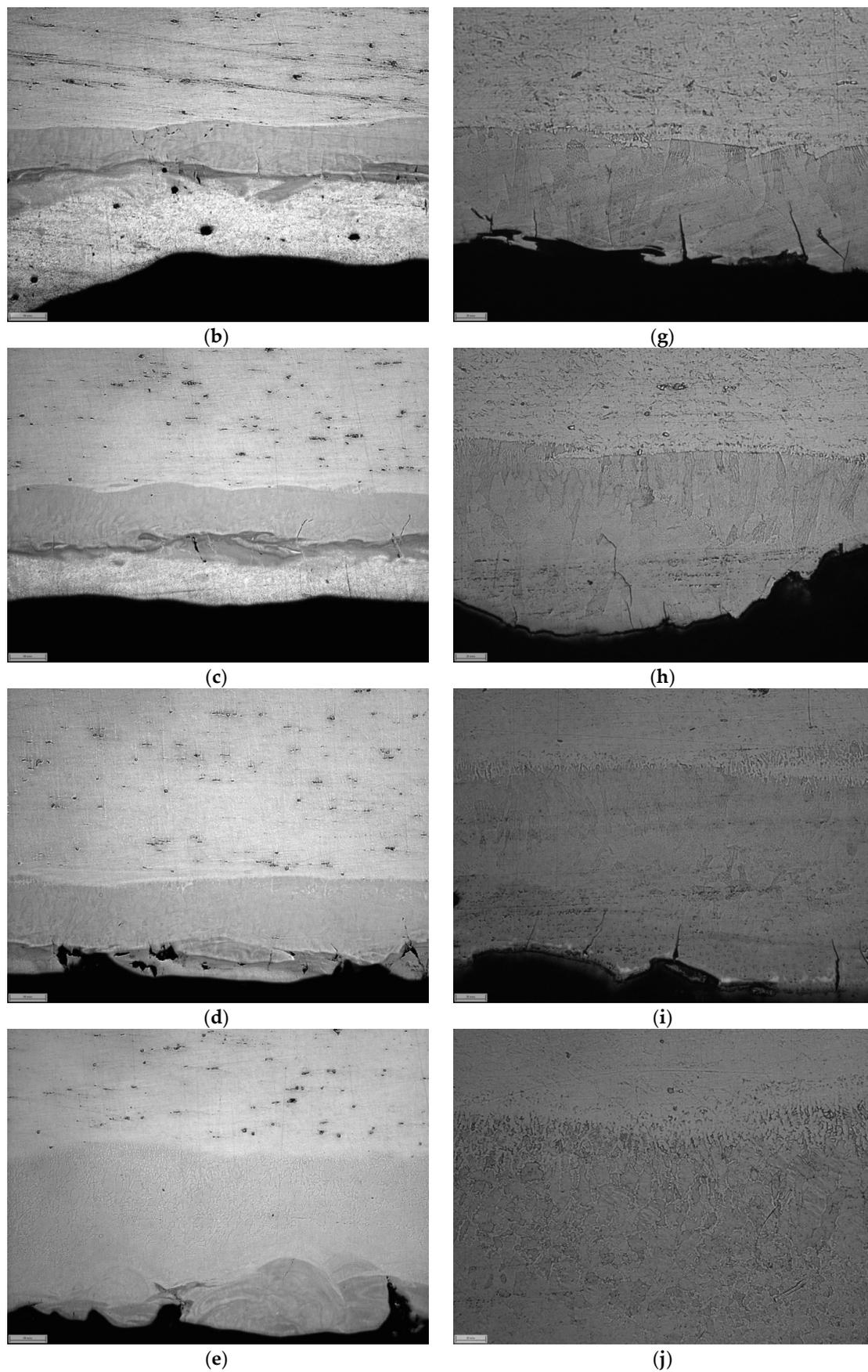
**Figure 4.** Microstructure of bimetal interface zone: (a,f) SLM scanning mode 1; (b,g) SLM scanning mode 2; (c,h) SLM scanning mode 3; (d,i) SLM scanning mode 4; (e,j) SLM scanning mode 5; (a–e) 200 $\times$ , without etching; (f–j) 500 $\times$ , after etching.
