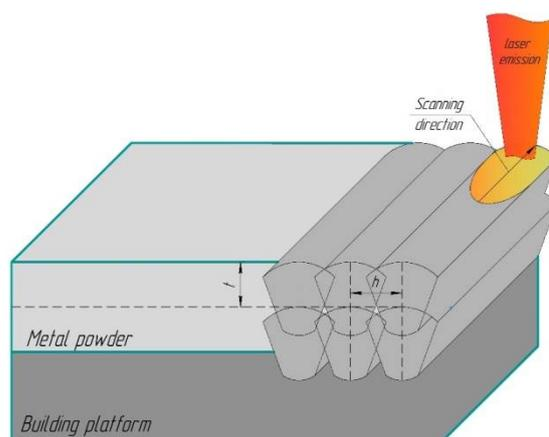
**Figure 2.** Selective laser melting (SLM) scanning parameters.
