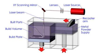
Figure 1. Typical Laser Powder Bed Fusion (L-PBF) process configuration.
