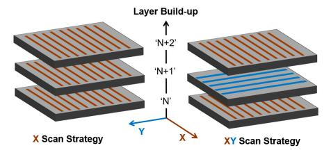
**Figure 5.** The bi-directional (X) and cross-directional (XY) scan strategies used by Becker et al. [39] and Bhardwaj et al. [38] to compare the residual stress state, texture, and mechanical properties in maraging steel 300. "*N*" represents an arbitrary build layer and subsequent layers are labelled "N + 1" and "N + 2".
