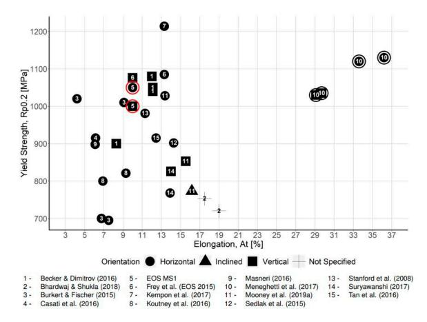
**Figure 6.** Comparison of the as-built yield strength (Rp0.2) and %elongation (At) properties by AM build-orientation for maraging steel 300 test-specimens fabricated using various geometries, processing parameters, scan strategies, and powder feedstock types.
