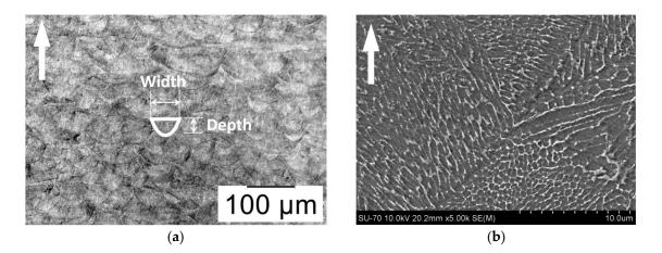
**Figure 4.** (a) Low magnification optical and (b) high magnification Scanning Electron Microscope (SEM) images of laterally sectioned structure fabricated with the EOS EOSINT M280 L-PBF system using the manufacturer's recommended set of parameters (MS1 Performance 2.0) and EOS maraging steel 300 powder (codified by EOS as MS1). The arrows indicate the additive manufacturing (AM) build direction.
