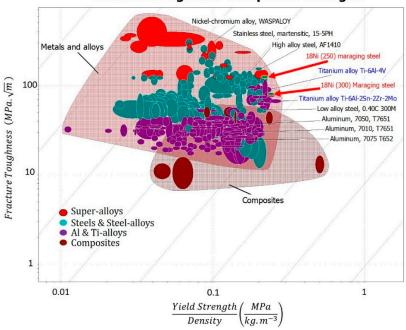
Fracture Toughness vs. Specific Strength
