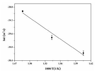
Figure 10. Growth constants for the reaction layers as a function of temperature.
