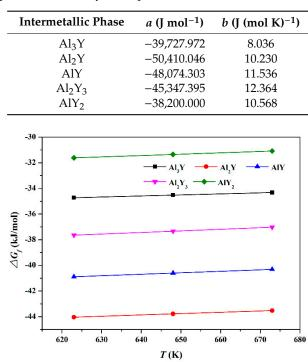
**Figure 6.** Gibbs energy of formation of Al-Y intermetallic phases in the temperature range of this experiment.
