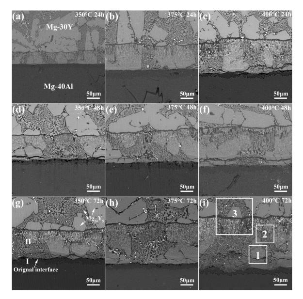
**Figure 1.** Back-scattered electron (BSE) micrographs of the diffusion couples annealing at 350, 375 and 400 °C for 24, 48 and 72 h. (a) at 350 °C, (b) at 375 °C and (c) at 400 °C for 24 h; (d) at 350 °C, (e) at 375 °C and (f) at 400 °C for 48 h; (g) at 350 °C, (h) at 375 °C and (i) at 400 °C for 72 h.
