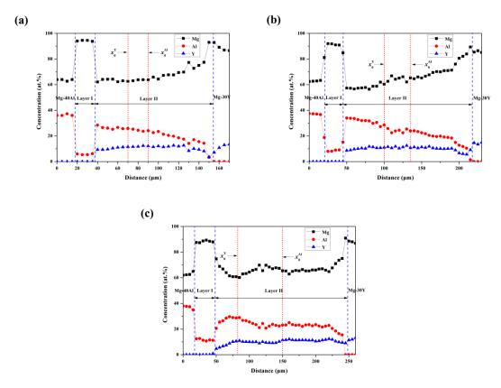
**Figure 2.** Concentration profiles Mg, Al and Y on the cross-section along the direction of diffusion for the diffusion couples annealed for 72 h at temperatures of (**a**) 350, (**b**) 375 and (**c**) 400 °C, respectively.  $x_0^{Al}$  and  $x_0^{Y}$  is the location of Matano plane for Al and Y, respectively.
