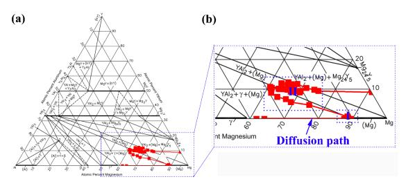
**Figure 3.** (a) The diffusion path for the diffusion couple on isothermal section at 400 °C of the Mg-Al-Y system, (b) a larger version of the dotted box in Figure 3a.
