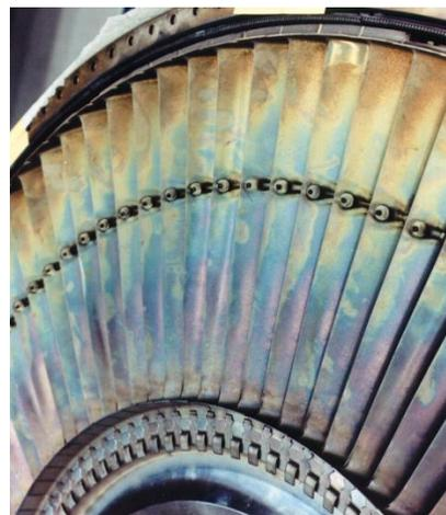
**Figure 12.** Image of the 747 class engine low-pressure turbine (LPT) rotor with Gamma alloy air foils after the demanding but successful factory test described earlier.
