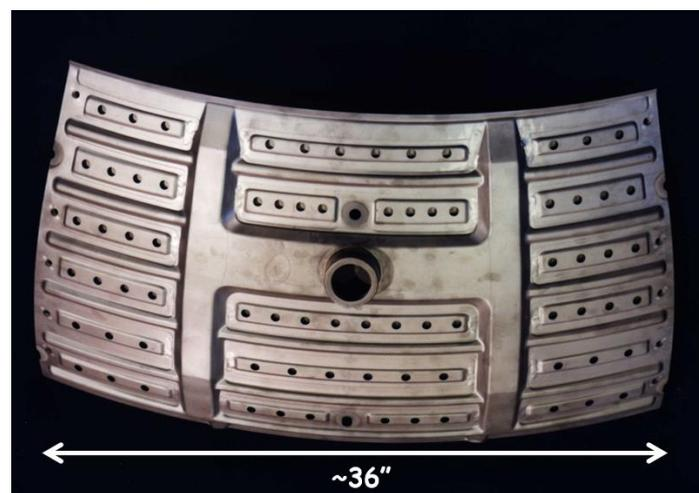
**Figure 3.** Example of a complex sheet metal engine part made by superplastic forming and diffusion bonding (SPFDB) [2].
