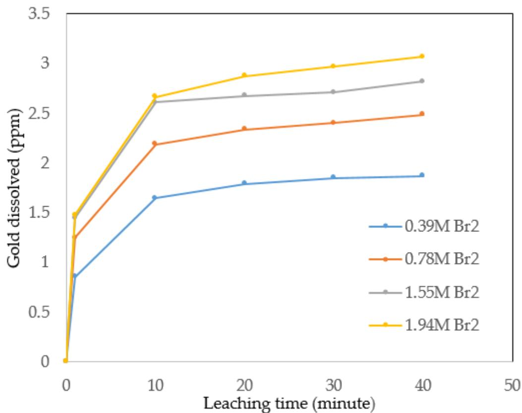
Figure S4. Effect of bromine concentration on gold dissolution at 23.5 °C and 400 RPM.
