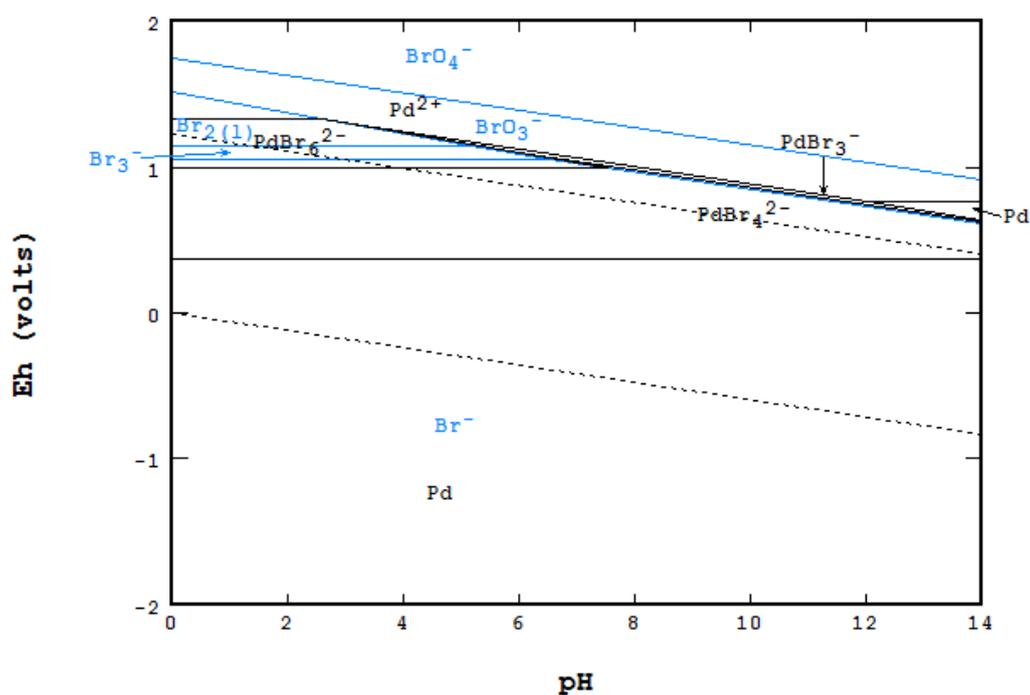
Figure S2. Eh-pH diagram of Br-Pd-H<sub>2</sub>O system at 25 °C ([Pd] = 10<sup>-5</sup> M, [Br] = 0.775M) (Stabcal).
