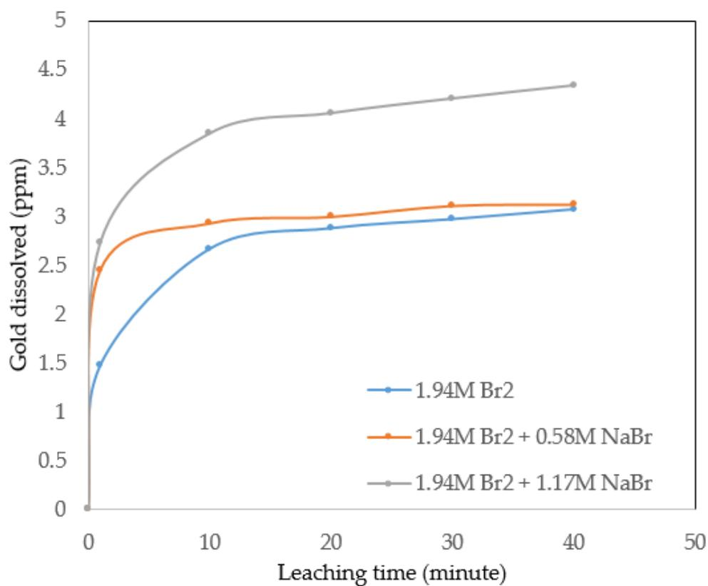
Figure S6. Effect of sodium bromide on gold dissolution at 23.5 °C and 400 RPM.
