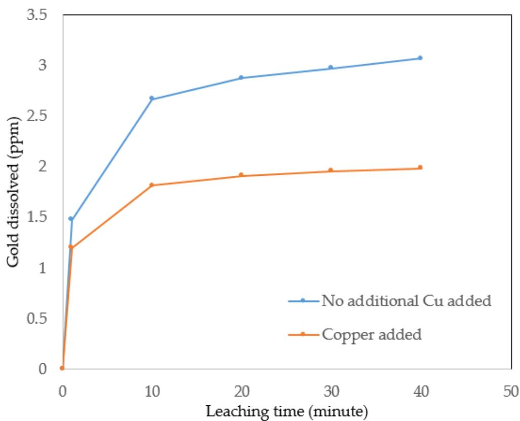
Figure S7. Effect of copper on gold dissolution at 23.5 °C and 400 RPM.
