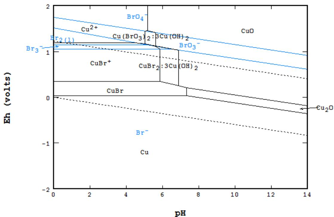
Figure S3. Eh-pH diagram of Br-Cu-H<sub>2</sub>O system at 25 °C ([Cu] = 10<sup>-3</sup> M, [Br] = 0.775M) (Stabcal).
