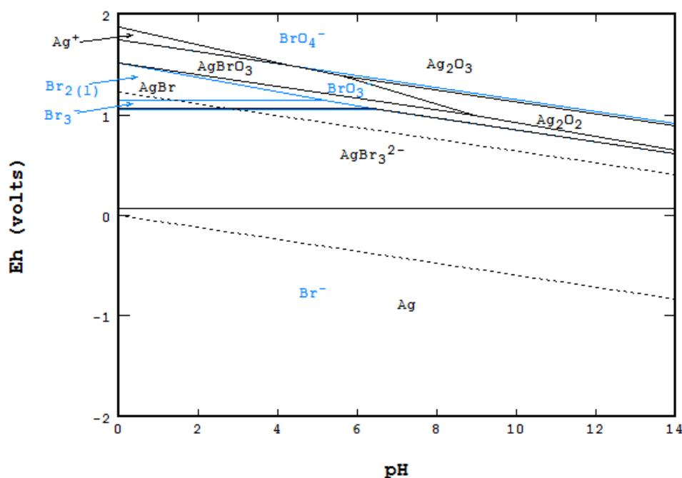
Figure S1. Eh-pH diagram of Br-Ag-H<sub>2</sub>O system at 25 °C ([Ag] = 10<sup>-4</sup> M, [Br] = 0.775M) (Stabcal).
