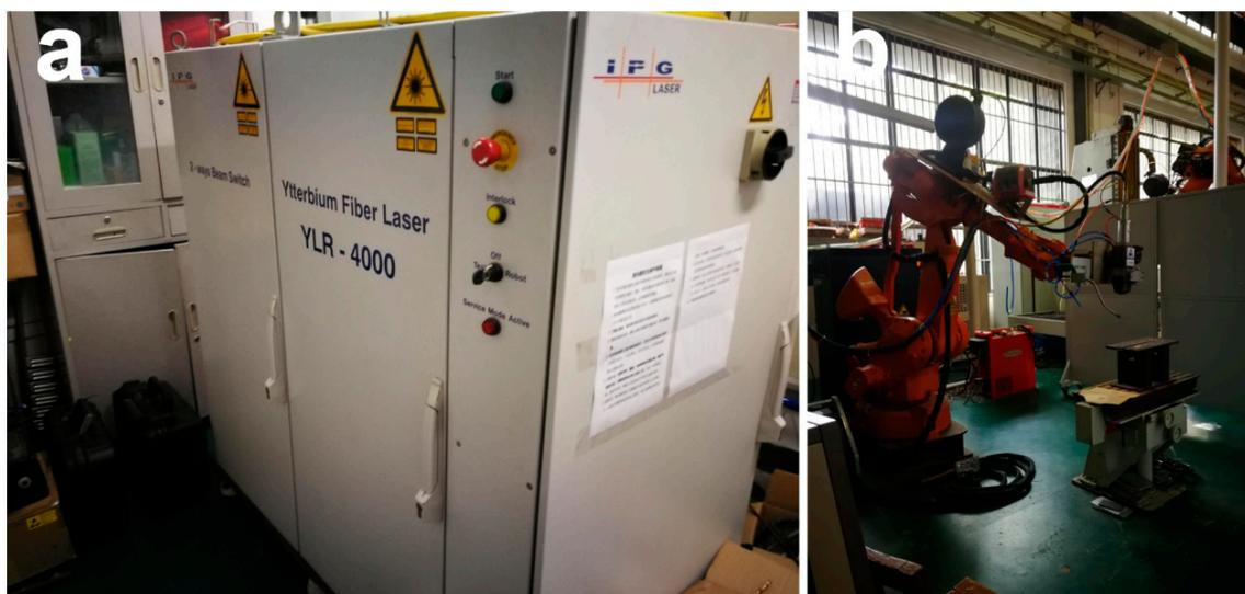
**Figure 5.** Welding devices: (a) IPG YLR-4000 fiber laser; (b) ABB IRB4400 robot.
