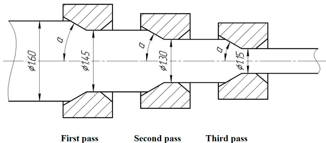
**Figure 2.** Schematic diagram of the multipass drawing process; unit: mm.
