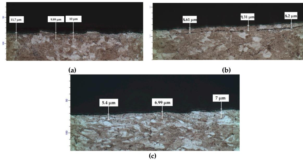
**Figure 3.** Thickness of fine grain layers after each pass of the multipass drawing process through  $\alpha = 4^\circ$  dies: (a) the first pass, (b) the second pass, (c) the third pass.
