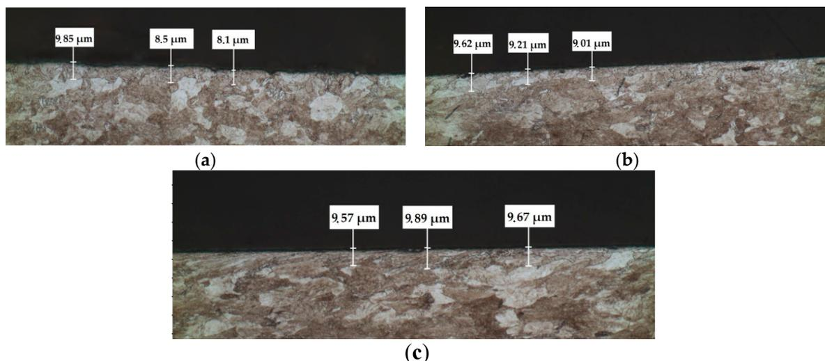
**Figure 6.** Thickness of the fine grain layers after each pass of the multipass drawing process through  $\alpha = 5^\circ$  dies: (a) the first pass, (b) the second pass, (c) the third pass.
