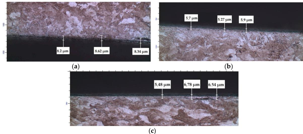
**Figure 5.** Thickness of the fine grain layers after each pass of the multipass drawing process through  $\alpha = 4^\circ$  dies: (a) the first pass, (b) the second pass, (c) the third pass.
