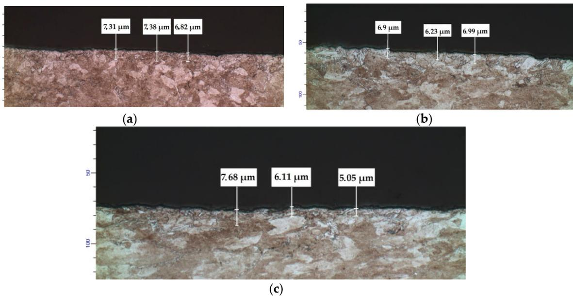
**Figure 4.** Thickness of fine grain layers after each pass of the multipass drawing process through  $\alpha = 5^\circ$  dies: (a) the first pass, (b) the second pass, (c) the third pass.
