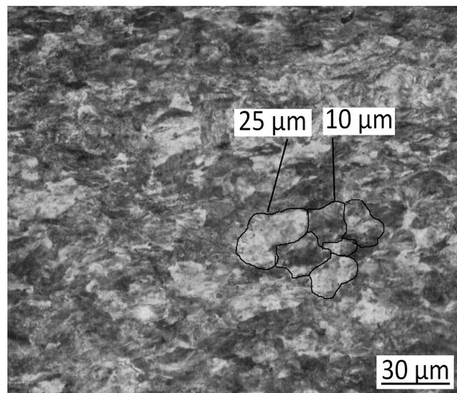
**Figure 1.** Microstructure of the wire material before multipass drawing,  $\times 1000$ .
