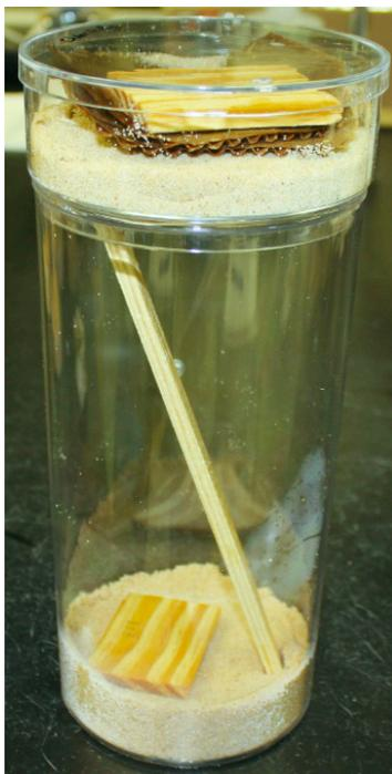
**Figure 1.** Bioassay arena showing top and bottom foraging sites connected with a ramp.
