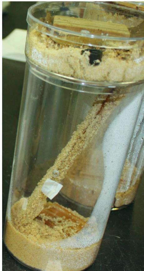
**Figure 3.** Shelter tube construction and termites on ramp at chlorantraniliprole 1 ppm treatment.
