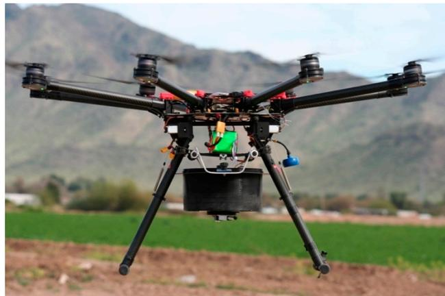
**Figure 1.** Photograph of the Hermes uncrewed aircraft system (UAS) used to release sterile codling moths in the Okanagan in 2016 and 2017. The UAS is shown in flight. The moth storage and release device is mounted under the airframe, between the landing gear.
