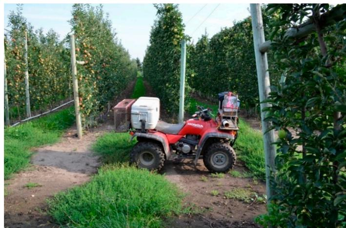
**Figure 2.** Photograph of a modified Honda Fourtrax all-terrain vehicle (ATV) used by the Okanagan–Kootenay Sterile Insect Release Program to release sterile codling moths (*Cydia pomonella*) in apple orchards. Moths are stored in a cooler on the rear of the ATV and released from the release device on the front of the vehicle (photograph by Tom Walker, 2015).
