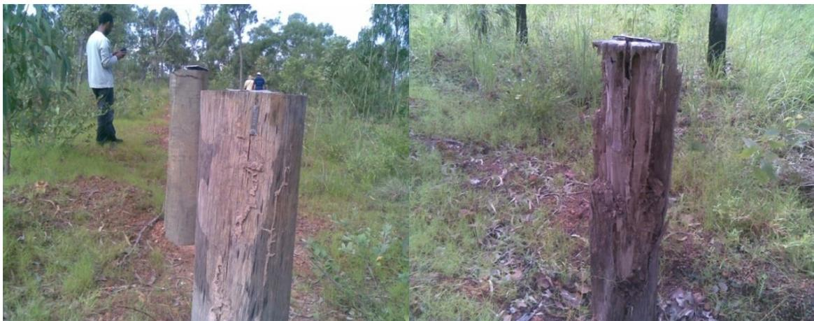
**Figure 9.** Untreated poles showing varying degrees of termite attack.
