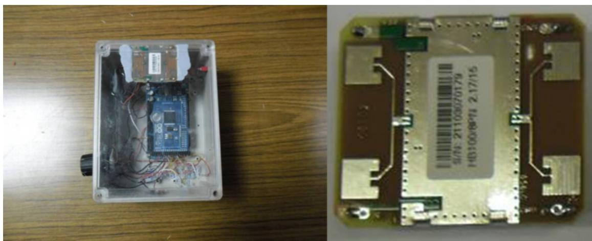
**Figure 8.** (Left) Sensor box with the HB100 radar module (right).
