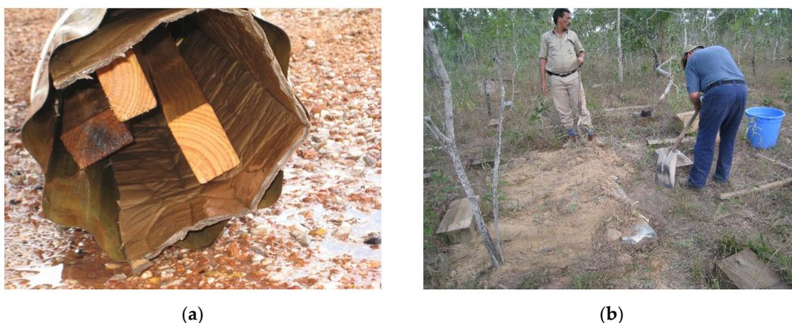
**Figure 3.** Termite bait station (a) during preparation and (b) being installed by the authors.
