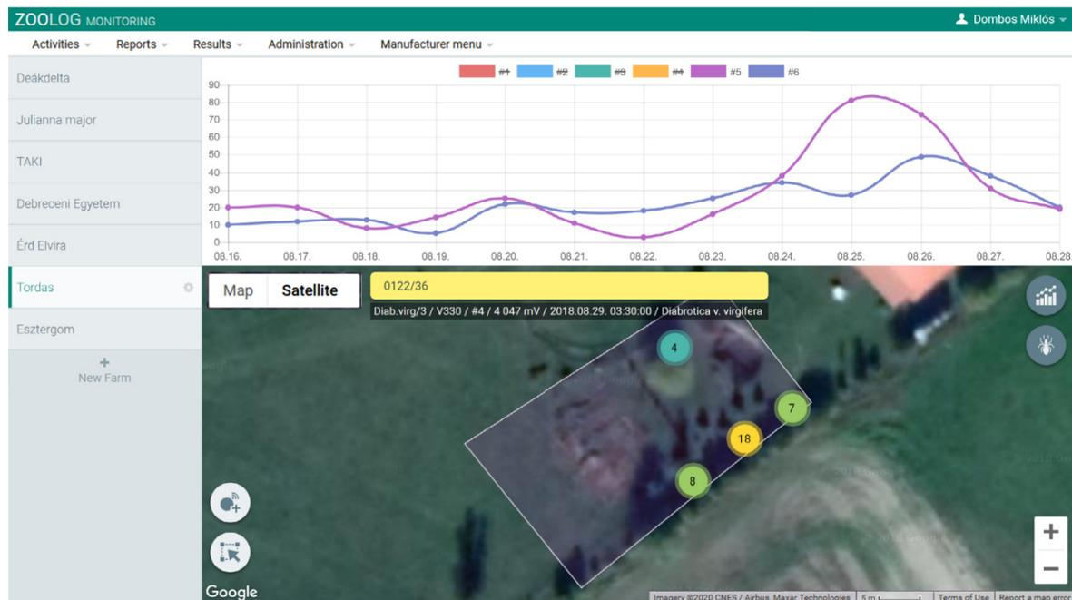
**Figure 2.** The ZooLog Online Web Interface: The monitoring system provides daily data via the internet. The probes and their status are visualized on a map. This interface is also used for setting the probes and data filtering. Results of the detection data can be downloaded and automatically visualized as graphs, typically the number of detected insects per day.
