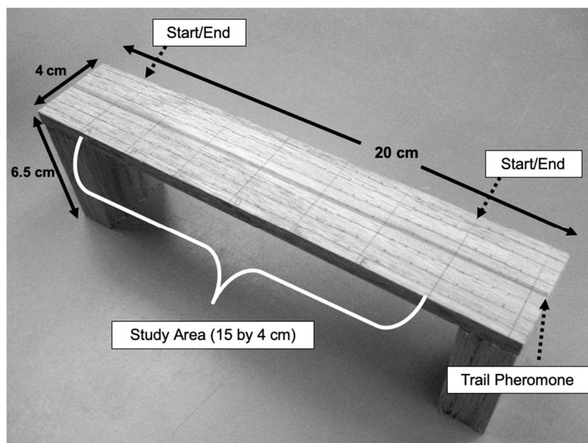
**Figure 1.** Wooden bridges (40 × 150 mm with 65 mm elevation from arena floor) used in trail-following arenas. Black lines and dots were spaced in a 5 × 5 mm grid and served as guides for measurements of ant movement in the study area, ant path deviations away from the longitudinal pheromone trail (amplitude), and quantification of the ant movement. A gray longitudinal band was added graphically to the picture to represent the centrally applied trail pheromone.
