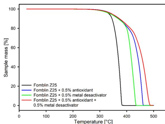
**Figure 7.** Temperature-dependent mass loss of Fomblin Z25 and its mixtures with additives.
