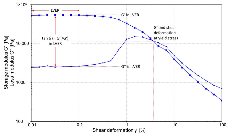
**Figure 1.** Depiction of a representative amplitude sweep and extractable output parameters.
