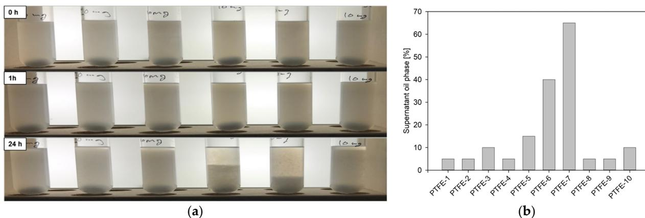
**Figure 4.** (a) Settling of dilute PFPE/PTFE dispersions at different times. (b) Calculated relative height of supernatant oil phase of sedimented dilute PFPE/PTFE dispersions.
