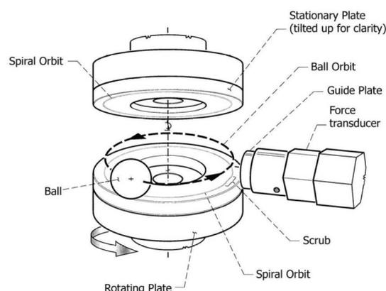
**Figure 2.** Schematic depiction of the spiral orbital tribometer (SOT) [33].
