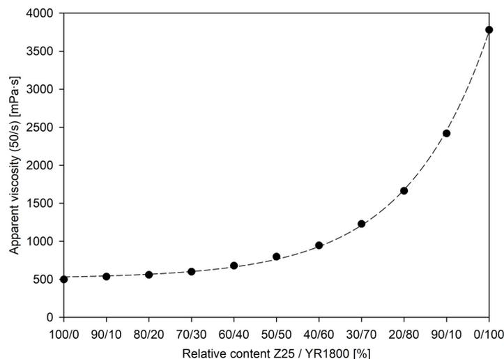
**Figure 3.** Viscosity of blends from Fomblin Z25 and Fomblin YR1800 at different compositions.
