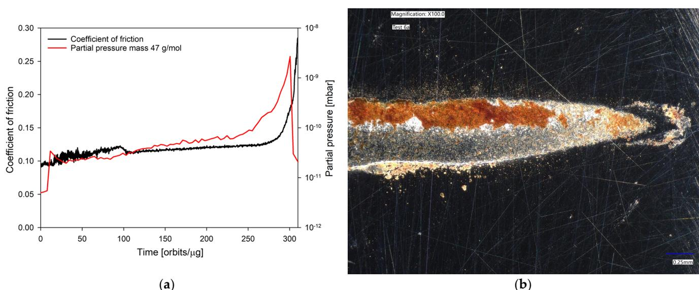
Figure 8. (a) Representative picture for evolution of coefficient of friction and partial pressure of a characteristic mass fragment 47 g/mol (CFO) during an SOT test with a PFPE lubricant. (b) Typical example of a wear scar showing the presence of lubricant degradation product (“brown sugar”).
