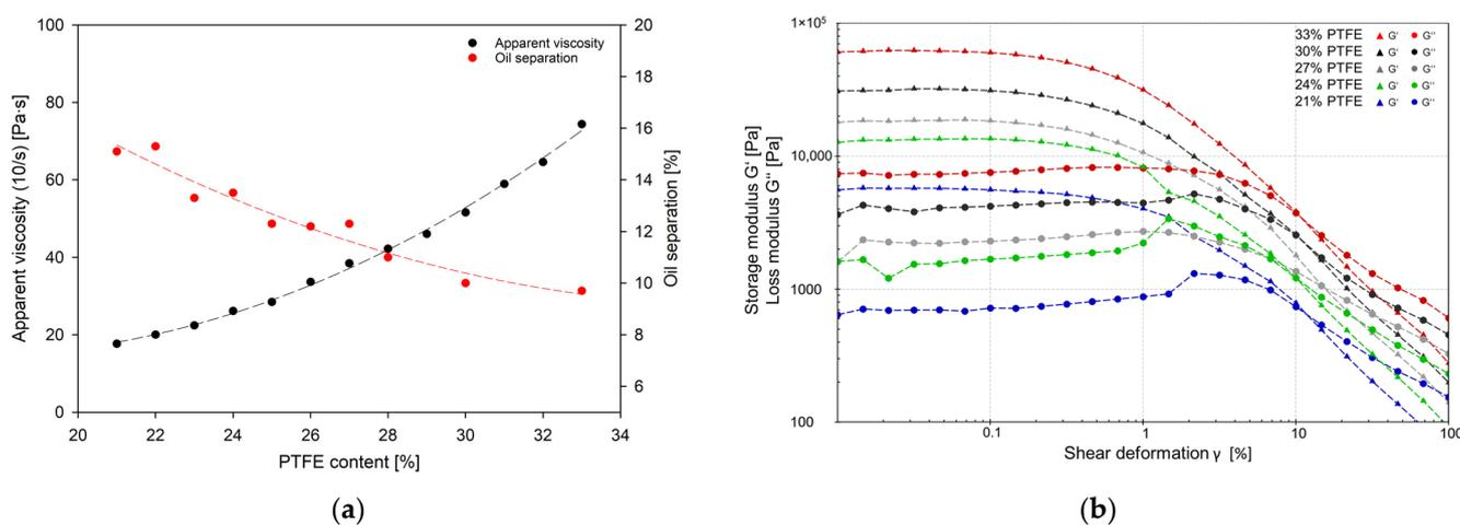
Figure 6. (a) Viscosity and oil separation of greases with different PTFE content. (b) Rheological amplitude sweeps of greases with different PTFE content.
