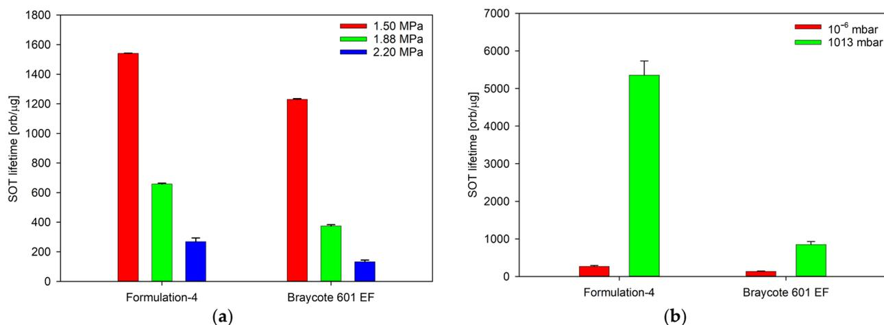
**Figure 9.** Comparison of tribological lifetimes from SOT test for formulation-4 and Braycote 601 EF (a) at different peak Hertzian contact pressure in high vacuum ( $10^{-6}$  mbar) and (b) at different pressure with a peak Hertzian contact pressure of 2.20 MPa.
