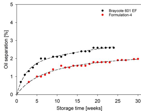
**Figure 10.** Results of long-term oil separation tests according to ASTM D6184 at room temperature for formulation-4 and Braycote 601 EF (dashed lines indicate trend).
