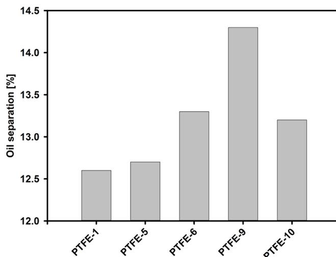
Figure 5. Oil separation of greases with different PTFE powders at 25% mass content and PFPE as base oil.
