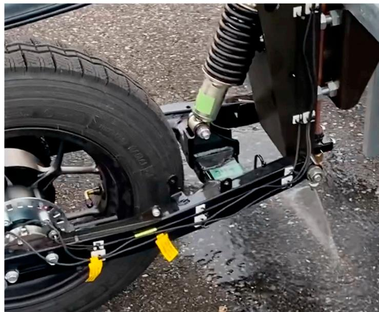
**Figure 7.** Sprinkler placed in front of measurement tire [32].
