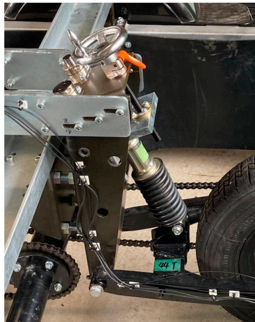
Figure 9. Load setting mechanism [32].
