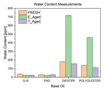
**Figure 8.** Water concentration of fresh, electrically aged (E\_Aged), and thermally aged (T\_Aged) base oils.
