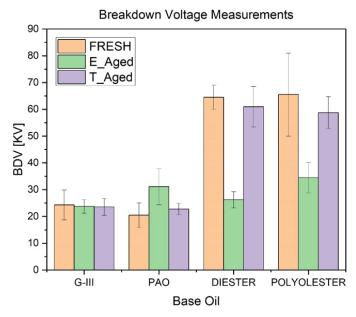
**Figure 7.** Breakdown voltage of fresh, electrically aged (E\_Aged), and thermally aged (T\_Aged) base oils.
