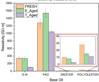
**Figure 6.** Resistivity of fresh, electrically aged (E\_Aged), and thermally aged (T\_Aged) base oils.
