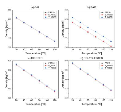
**Figure 2.** Density of fresh, thermally aged, and electrically aged samples: (**a**) G-III, (**b**) PAO, (**c**) diester, (**d**) polyolester.
