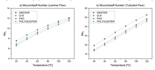
Figure 4. Mouromtseff number of fresh samples in (a) laminar flow; (b) turbulent Flow.
