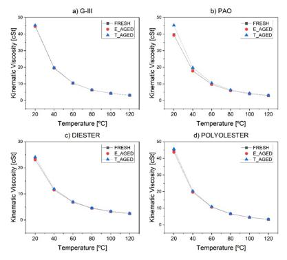
**Figure 1.** Kinematic viscosity of fresh, thermally aged, and electrically aged samples: (a) G-III, (b) PAO, (c) diester, (d) polyolester.
