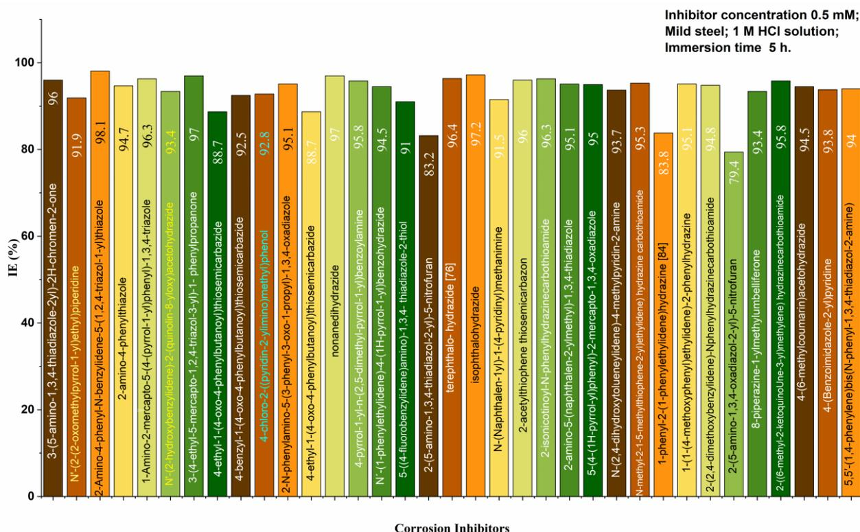
**Figure 11.** Comparison between several synthesized organic corrosion inhibitors.
