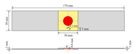
Figure 1. Dimensions and overlap type of copper sheets.
