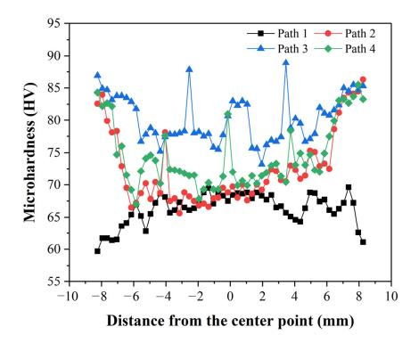
Figure 9. Cross-sectional microhardness of the welded joints under the different tool plunging paths.
