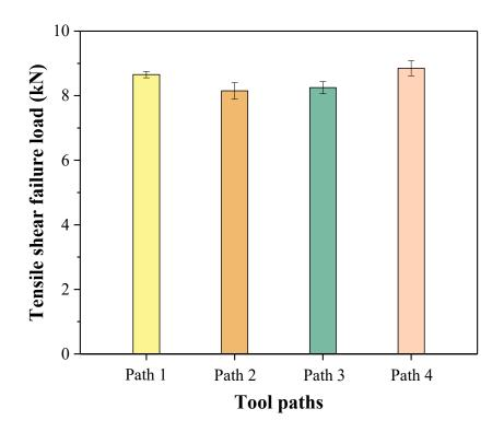
Figure 10. Tensile shear failure loads of the welded joints under different tool plunging paths.
