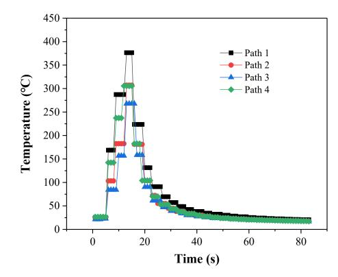
Figure 8. Welding temperature under different tool plunging paths.
