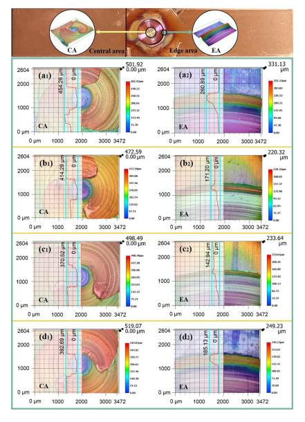
**Figure 5.** Appearance features of the welded joints under path 1 ( $a_1$ , $a_2$ ), path 2 ( $b_1$ , $b_2$ ), path 3 ( $c_1$ , $c_2$ ), and path 4 ( $d_1$ , $d_2$ ).
