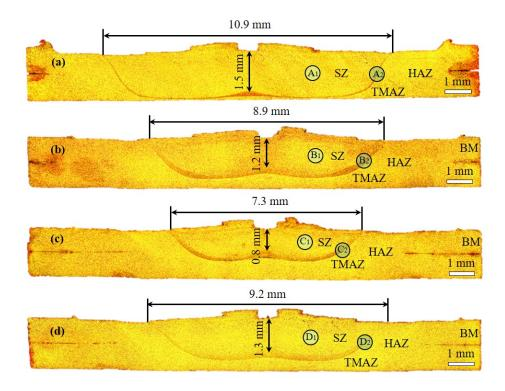
**Figure 6.** Cross-sectional morphologies of the welded joints under path 1 (**a**), path 2 (**b**), path 3 (**c**), and path 4 (**d**).
