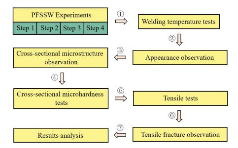
Figure 4. Flowchart of the research process.
