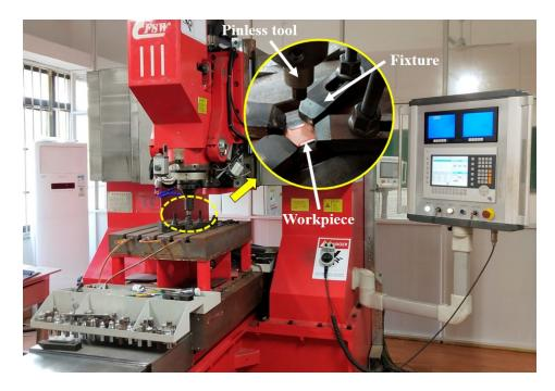
Figure 2. Photograph of the experimental platform.
