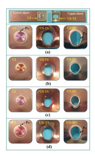
Figure 11. Fracture pictures of welded joints under path 1 (a), path 2 (b), path 3 (c), and path 4 (d).
