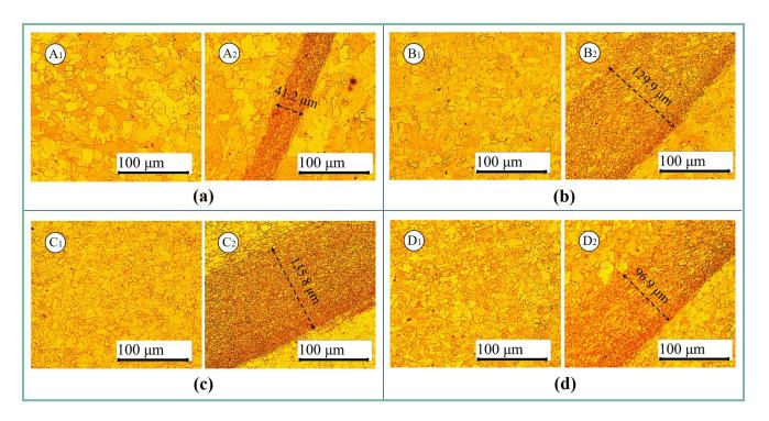
the stirring zone were larger and the width of the thermal-mechanical-affected zone was the smallest.
