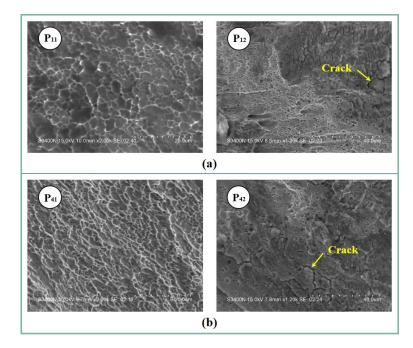
Figure 12. SEM morphologies of the welded joint fractures of path 1 (a) and path 4 (b).
