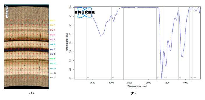
Figure 6. ATR-FTIR (a) measurement points, (b) spectrum—bands of interest (description in Table 4).
