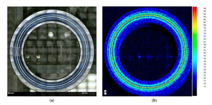
**Figure 4.** (a) Mosaic image with definition of the areas on the sample surface (1 = outside the raceway, 2 = outer raceway, 3 = middle of the raceway, 4 = inner raceway). (b) Corresponding element distribution colored as absolute intensities (0 to 100).
