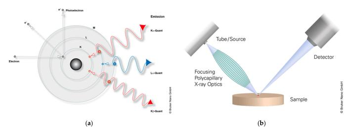
**Figure 3.** (a) Excitation of X-ray fluorescence radiation. (b) Schematic diagram of µXRF, M4 Tornado (Images courtesy of Bruker Nano GmbH).
