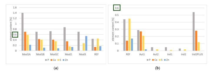
**Figure 7.** Comparison surface element concentrations of outer raceway: (**a**) model oils; (**b**) fully formulated.
