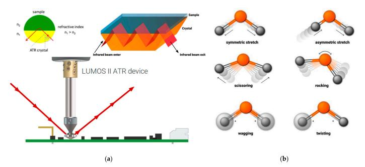
**Figure 5.** (a) Schematic diagram of ATR crystal. (b) Example of infrared vibration modes (images courtesy of Bruker Optics GmbH).
