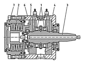
**Figure 1.** FE8 test rig setup [40]: 1—test bearing, 2—spring package, 3—shaft, 4—bearing housing drive side, 5—bearing housing spring side, 6—housing, 7—cup.
