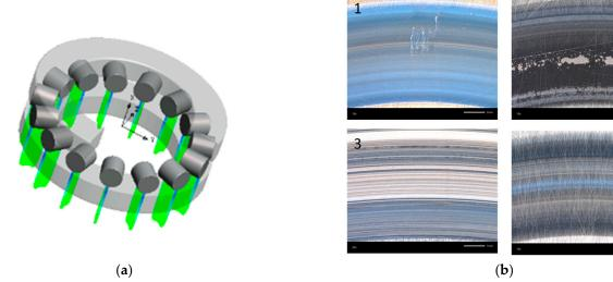
**Figure 2.** (a) FE8 test bearing load distribution; (b) washer images of results (1—WEC, 2—SIF, 3—wear, 4—no failure, suspended).
