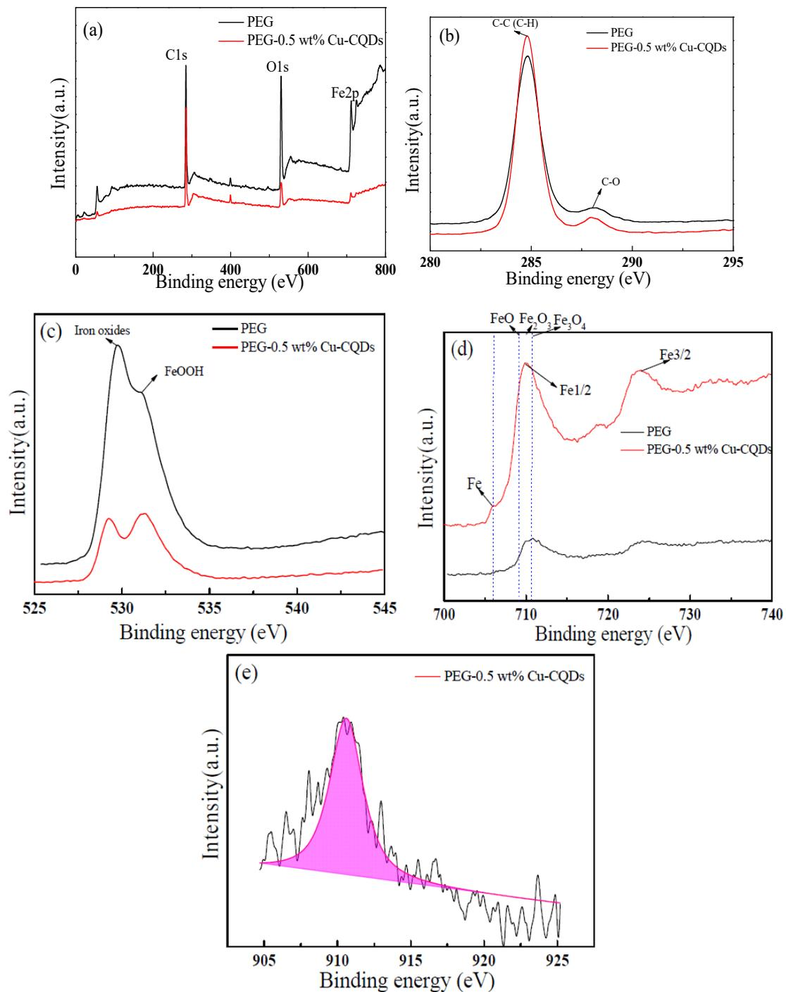
**Figure 10.** Valence analysis of different elements in the wear scar region of steel ball: (a) XPS total spectrum; (b) C1s; (c) O1s; (d) Fe<sub>2p</sub>; and (e) Cu<sub>2p</sub>.
