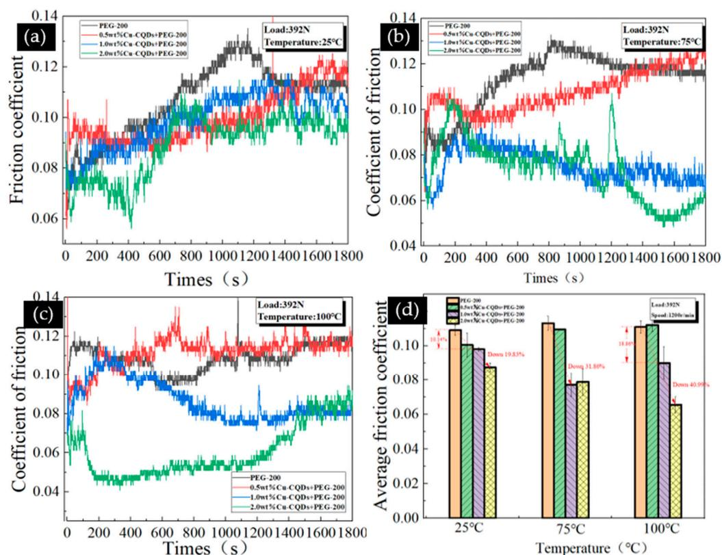
**Figure 4.** The changes of friction coefficients with different mass fractions of Cu-CQDs dispersion (1200 rpm/min, each group lasts for 30 min), (a) 25 °C; (b) 75 °C; (c) 100 °C; and (d) histogram of average friction coefficient under different working conditions.
