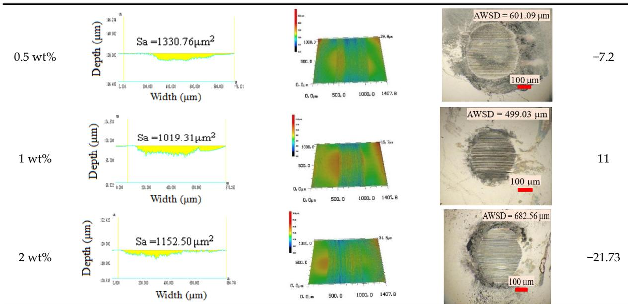
Figure 7. Cross-sectional area, three-dimensional morphology, average wear scar diameter, and change rate of wear scar area lubricated by different oil samples at 75 °C.
