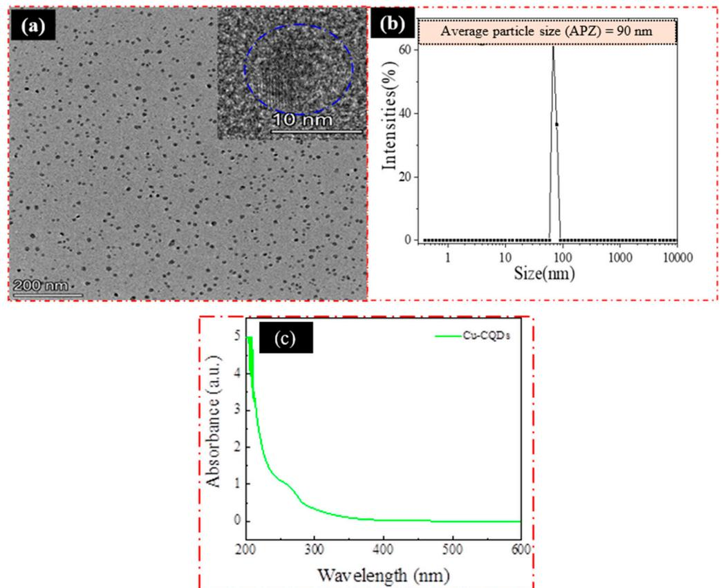
**Figure 2.** HRTEM, particle size distribution of Cu-CQDs in water and UV absorption spectrum of copper-doped carbon quantum dots. (a) TEM images of Cu-CQDs; (b) particle size distribution of Cu-CQDs in water; and (c) ultraviolet visible absorption spectrum.
