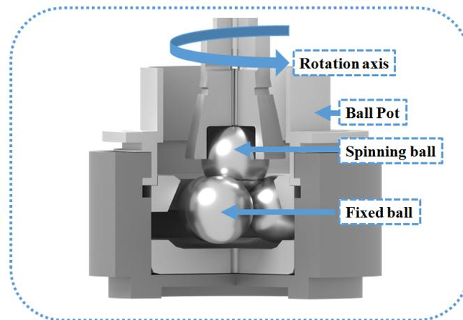
**Figure 3.** Schematic diagram of a four balls tribo-meter.
