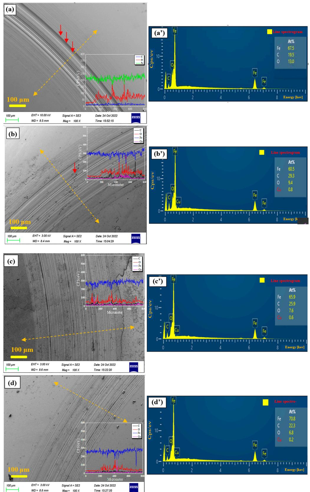
**Figure 9.** Surface wear scar morphology and energy spectrum analysis of steel ball lubricated by different content of copper-doped carbon, (a,a') pure PEG, (b,b') 0.5 wt% Cu-CQDs, (c,c') 1.0 wt% Cu-CQDs, and (d,d') 2.0 wt% Cu-CQDs.
