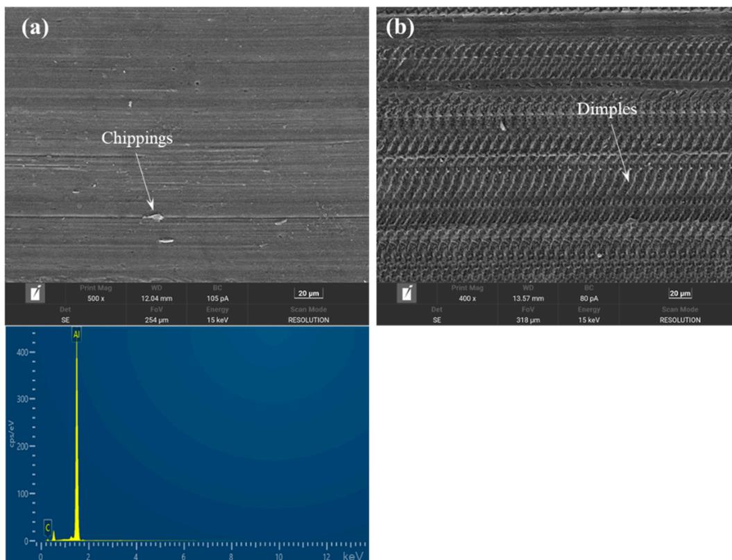
**Figure 7.** SEM images of the surface morphology of (a) CT and (b) UVAT processes under dry cutting conditions and the EDS results of the chipping in (a).
