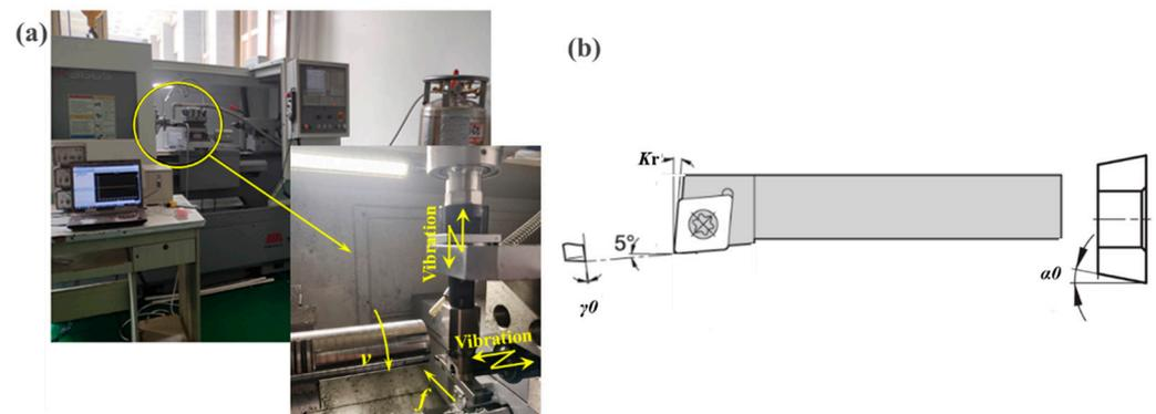
**Figure 2.** (a) Experimental equipment of the UVAT and NMQL method and (b) the cutting tool angles.
