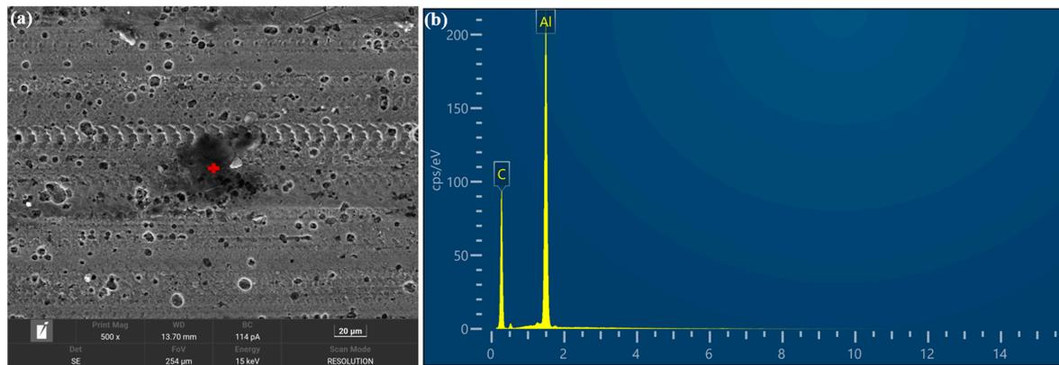
**Figure 5.** (a) SEM and (b) EDS images of the surface morphology of the UVAT and GN-MQL method.
