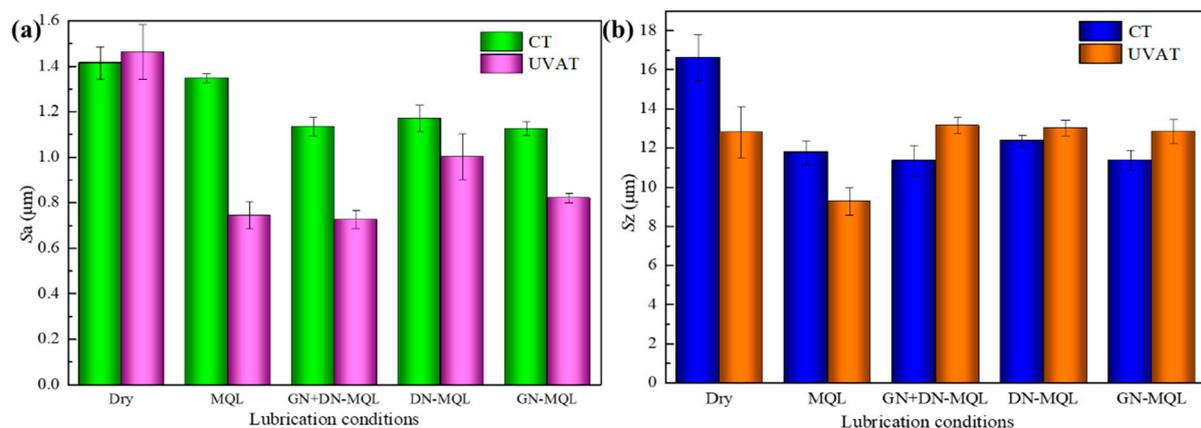
**Figure 6.** Areal surface roughness, (a)  $S_a$  and (b)  $S_z$ , of different cutting conditions.
