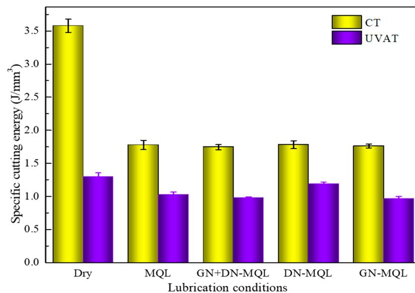
**Figure 3.** Specific cutting energy of different cutting conditions.
