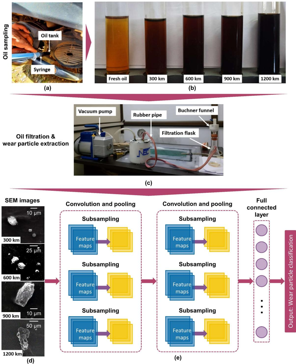
**Figure 1.** (a) Sampling lubricant from the engine, (b) lubricating oil samples after various intervals, (c) lubricant sample filtration setup, (d) representative SEM images of wear particles after various intervals, and (e) schematic of an image-processing CNN.
