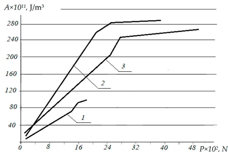
**Figure 5.** Physical interpretation of the integral parameter for assessment of the tribological properties of lubricants: 1—ISO-L-HM hydraulic oil; 2—engine oil SAE 5W-30, API CH; 3—gear oil SAE 75W-90, API GL-5.
