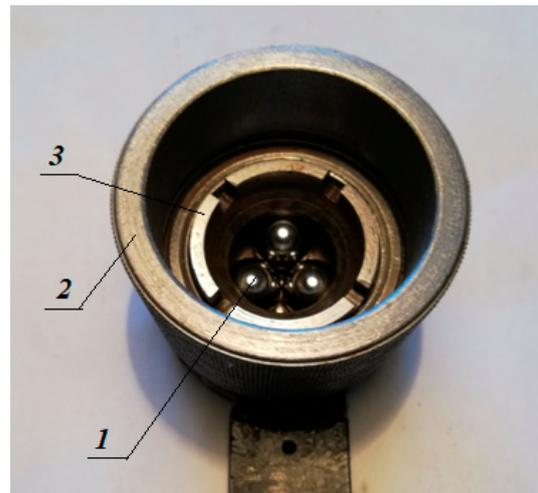
**Figure 2.** External view of the four-ball assembly. 1—fixed lower balls; 2—a glass for a lubricant to be tested; 3—nut for fixture of the three lower balls.
