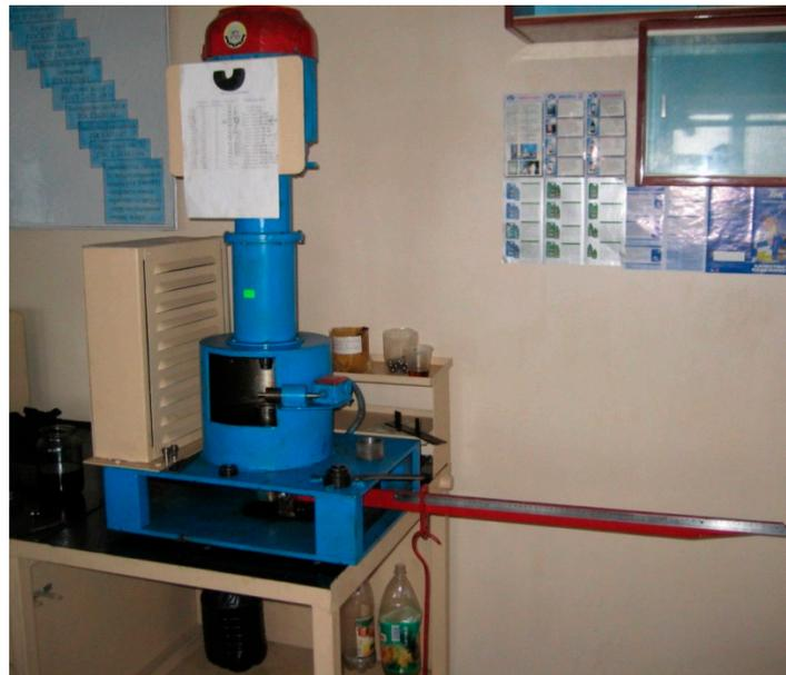
**Figure 3.** External view of a four-ball tribometer.
