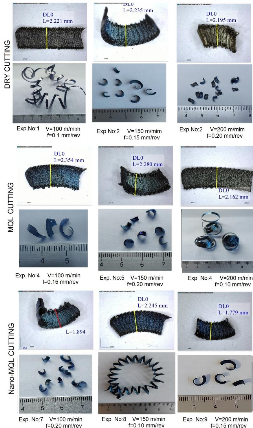
Figure 15. Chip morphology under dry, MQL, and nano-MQL cutting conditions.
